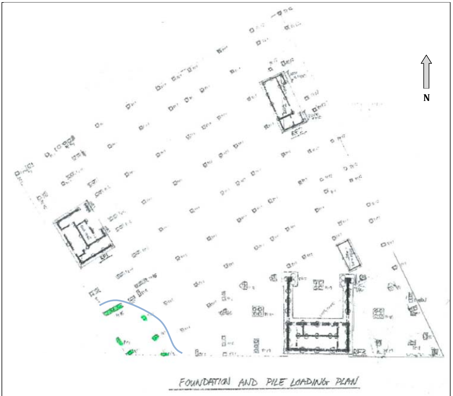
Figure 6: Foundation and piling plan. Approximate areas proposed for testing indicated in green. Proposed testing locations are indicative only and to be confirmed on site depending on location of existing services or other obstructions. Approximate area of original shoreline indicated by blue line. Reclaimed land to the east of blue line.
