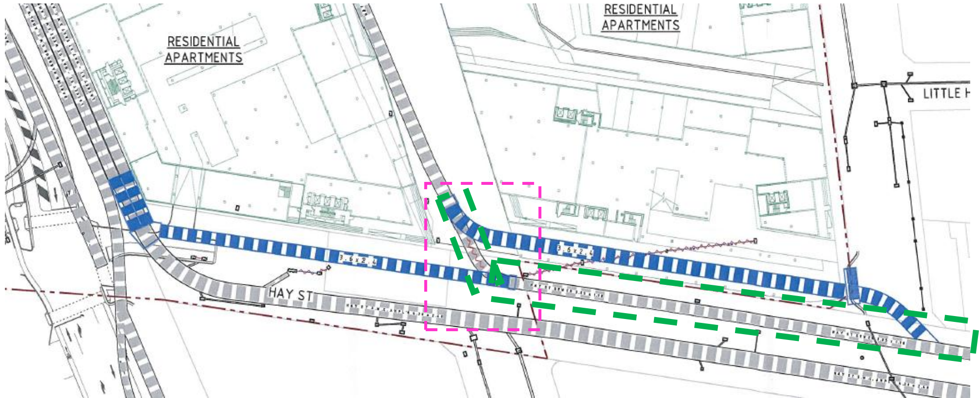
Figure 6: Plan showing works associated with new proposed culverts (blue) and adjustments to the heritage Hay Street Stormwater Channel. The green dashed line shows the location of the heritage listed Hay Street stormwater channel. The pink box indicates the proposed location of new culverts which are part of SSDA5.
