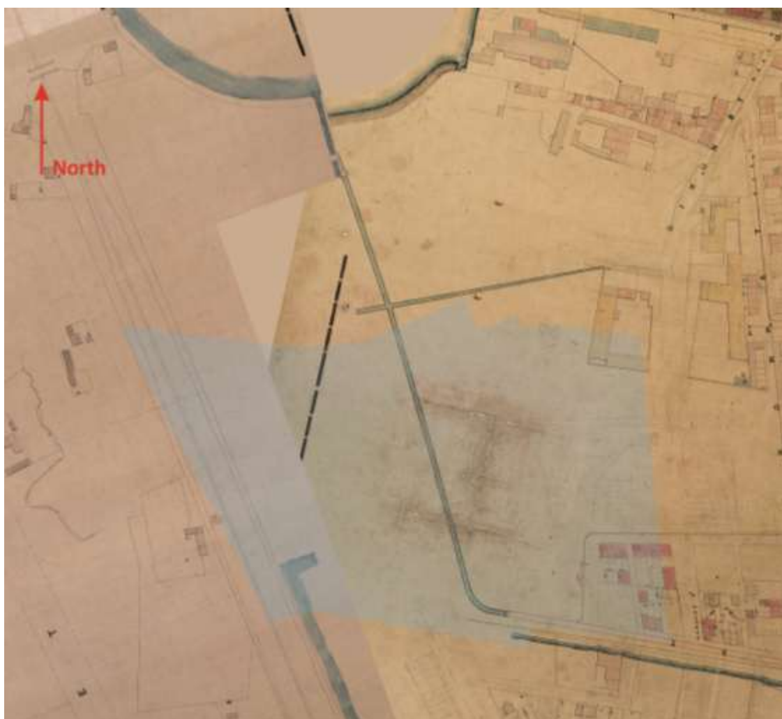
Figure 2.30: Part of the 1865 survey showing the reclamation of land at the head of Darling Harbour and the line of sewerage and stormwater channels draining into the harbour. The Hay Street sewer extension is the channel running approximately north-south and left open for a period of time. Note the pencil markings indicating the Council annotations of later buildings and streets. The former creekline and proposed drain along Hay Street to the south is visible. Trig Survey: Section T, 1865, Historical Atlas of Sydney, City of Sydney Archives.
