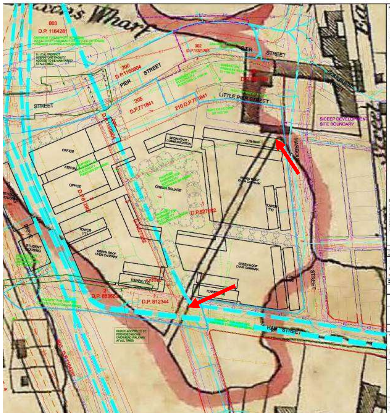
Figure 3.5: Overlay of services onto the 1854 plan showing dam wall (red arrows) to Dickson's millpond. Two large culverts cross through it along Hay Street. It is also likely that the high voltage cable near the northern red arrow has also cut through it. Rygate's overlay onto Woolcott & Clark's 1854 plan.
