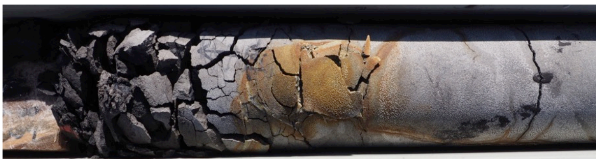
Plate 7 – Iron staining and sulphate salts due to partial oxidation of pyrite in a fracture. Hole SMC032, depth 174.3 m.
