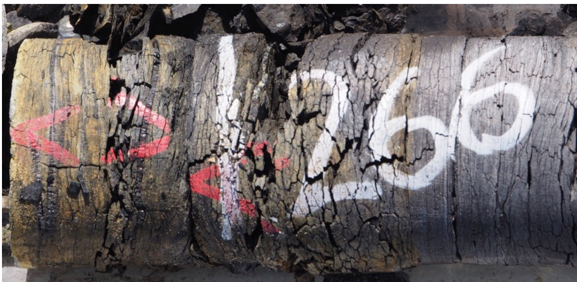
Plate 8 – Iron staining and sulphate salts due to partial oxidation of a pyritic zone. Hole SMC032, depth 265.95 to 266.10 m.
