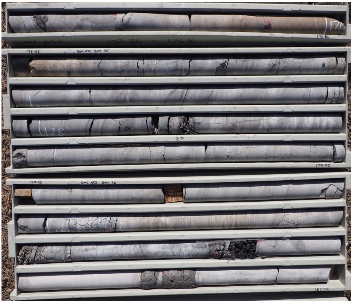
Plate 1 – Typical benign sandstone and siltstone overburden/interburden. Hole SMC032, depth 175.10 to 183.79 m.
