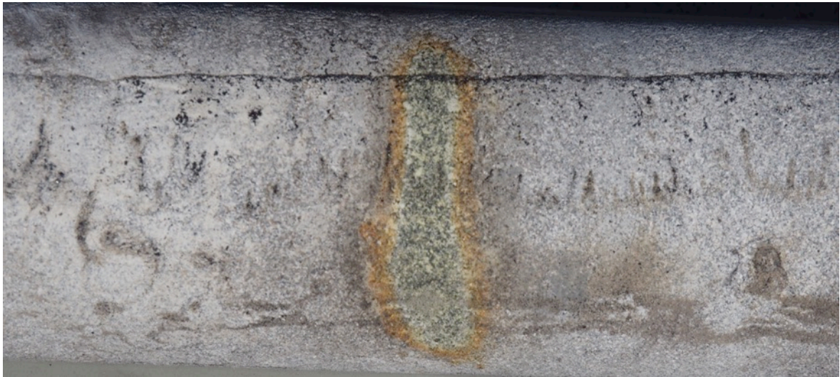
Plate 4 – Iron staining and sulphate salts due to partial oxidation of a pyrite containing lensoid in sandstone. Hole SMC032, depth 250.4 m.
