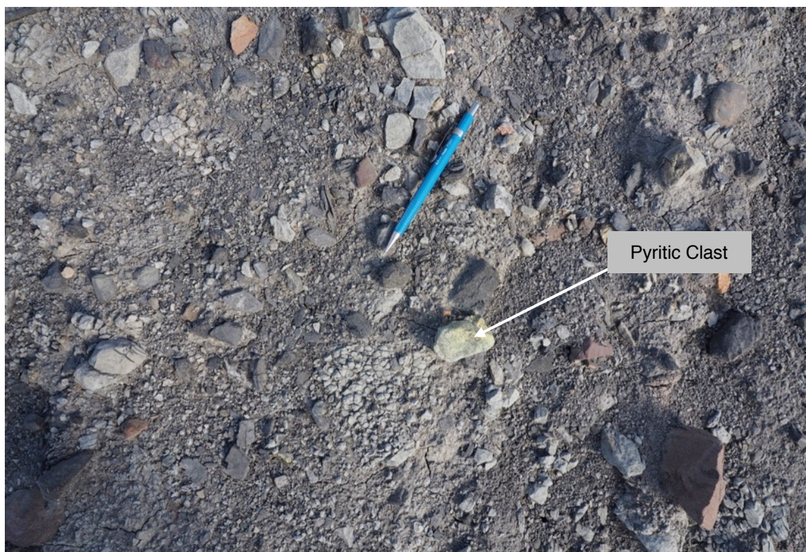
Plate 14 – Rejects placed in the Mount Owen North Pit showing isolated partly oxidised pyritic clast.
