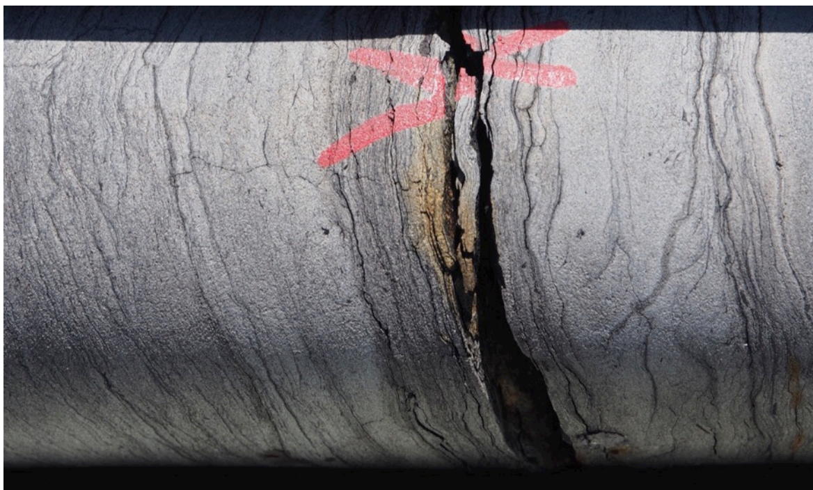
Plate 2 – Iron staining and sulphate salts due to partial oxidation of a pyrite coating parallel to bedding. Hole SMC032, depth 156.85 m.
