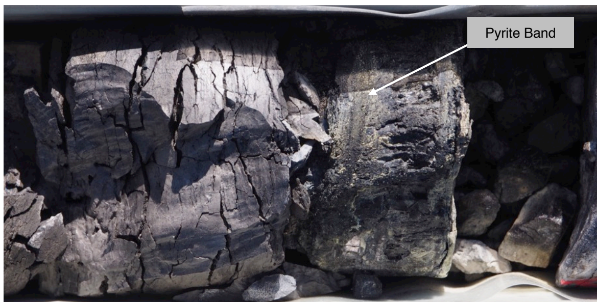
Plate 9 – Pyrite band (partly oxidised) parallel to bedding. Hole SMC032, depth 153.5 m.
