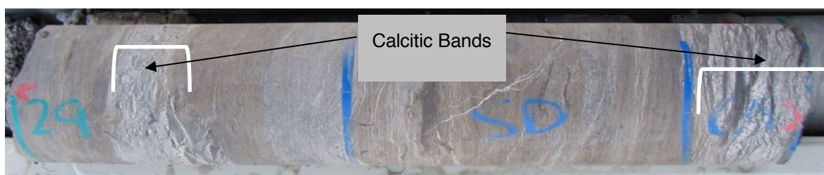
Plate 11 – Calcitic bands with cone-in-cone texture within a sideritic layer. Hole SMC001, 29.15 m depth.
