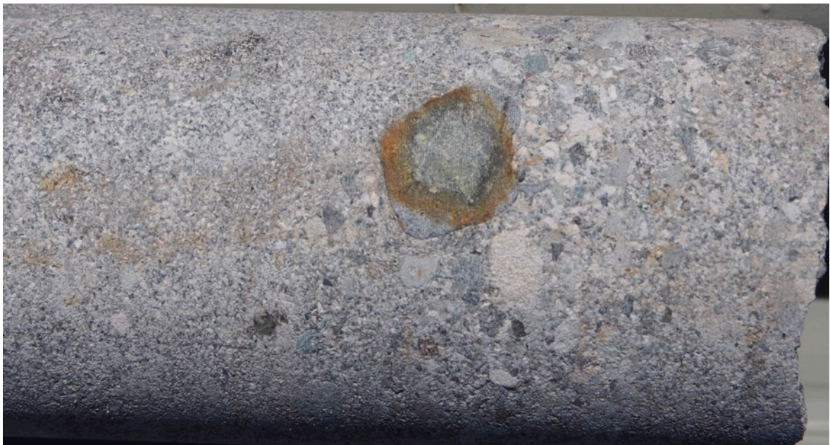
Plate 5 – Iron staining and sulphate salts due to partial oxidation of pyrite in a conglomerate clast. Hole SMC032, depth 192.1 m.
