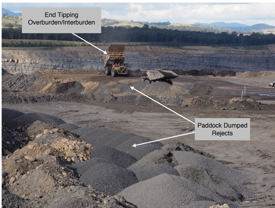
Plate 13 – End tipping of overburden/interburden and paddock dumping of rejects in the Mount Owen North Pit.
