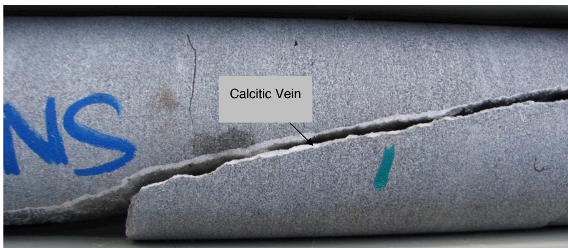
Plate 10 – Sandstone with calcitic carbonate in the matrix and veins. Hole SMC001, 51.5 m depth.
