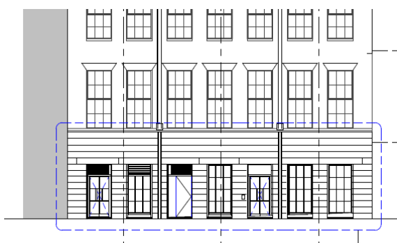
Figure 18 Beneficial House—Wynyard Lane elevation—showing proposed changes to the rear lane façade associated with the new stair and lift. (Source: Make + Architectus, A-285-20-32-1, 17 May 2019)
