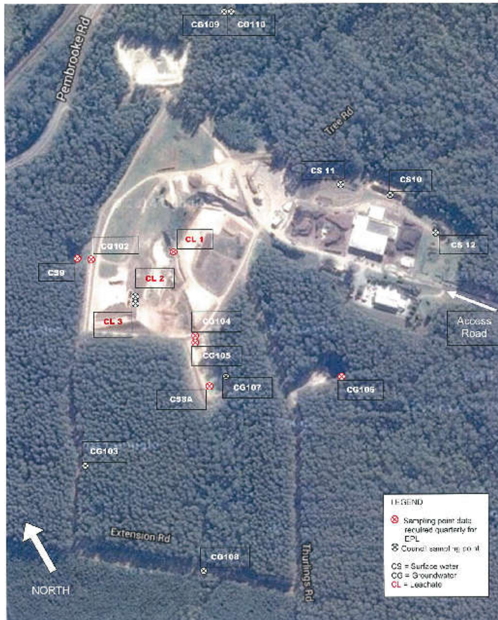
Cairncross Landfill - Bore and Surface Water Monitoring Point Locations
