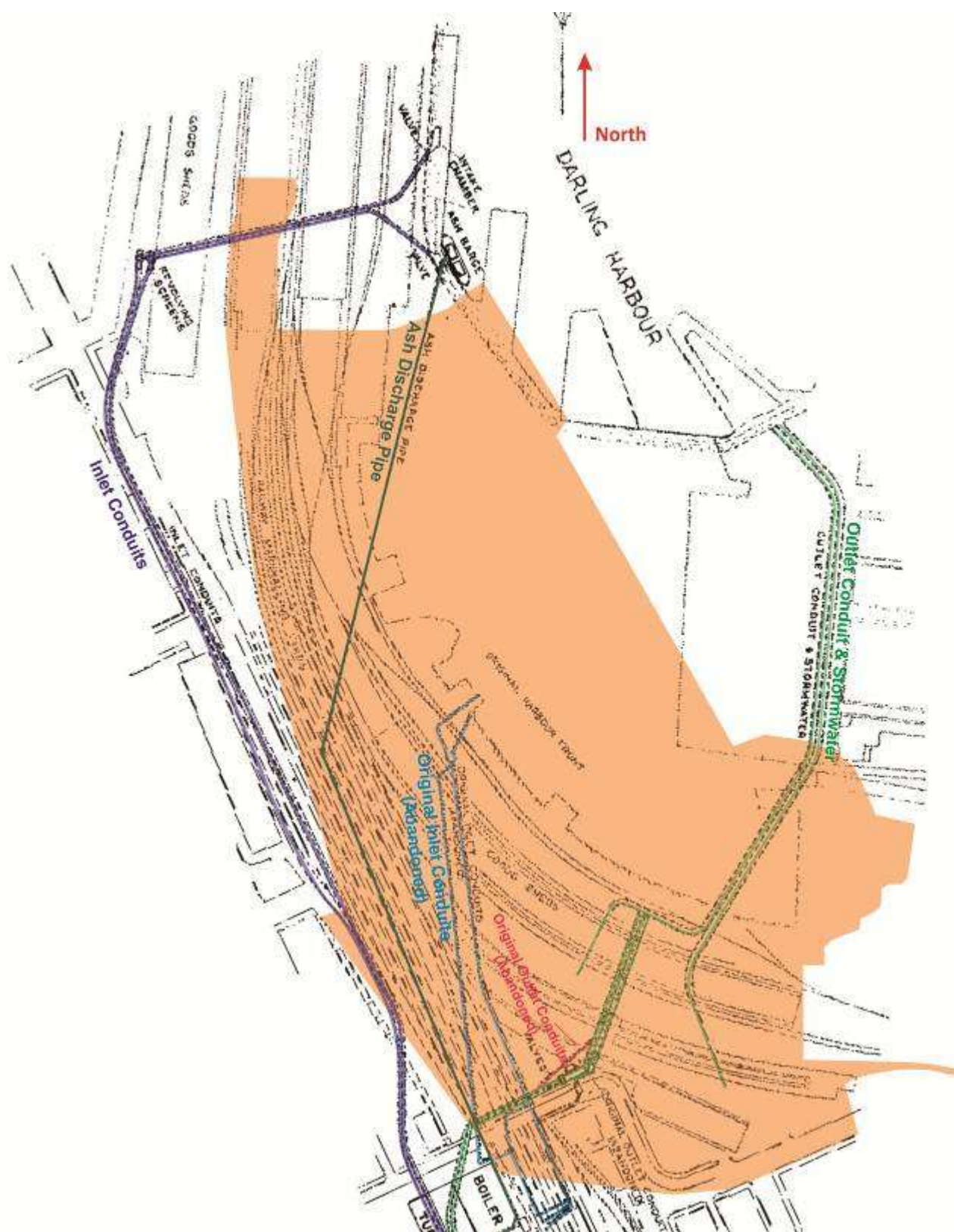
Figure 2.44: Plan showing the shoreline in relation to circulating water ducts and conduits inlets and outlet used in 1899 and those constructed in the mid 1920s. The location of intake sumps, valves and screens is also shown. Myers 1933: 255.
