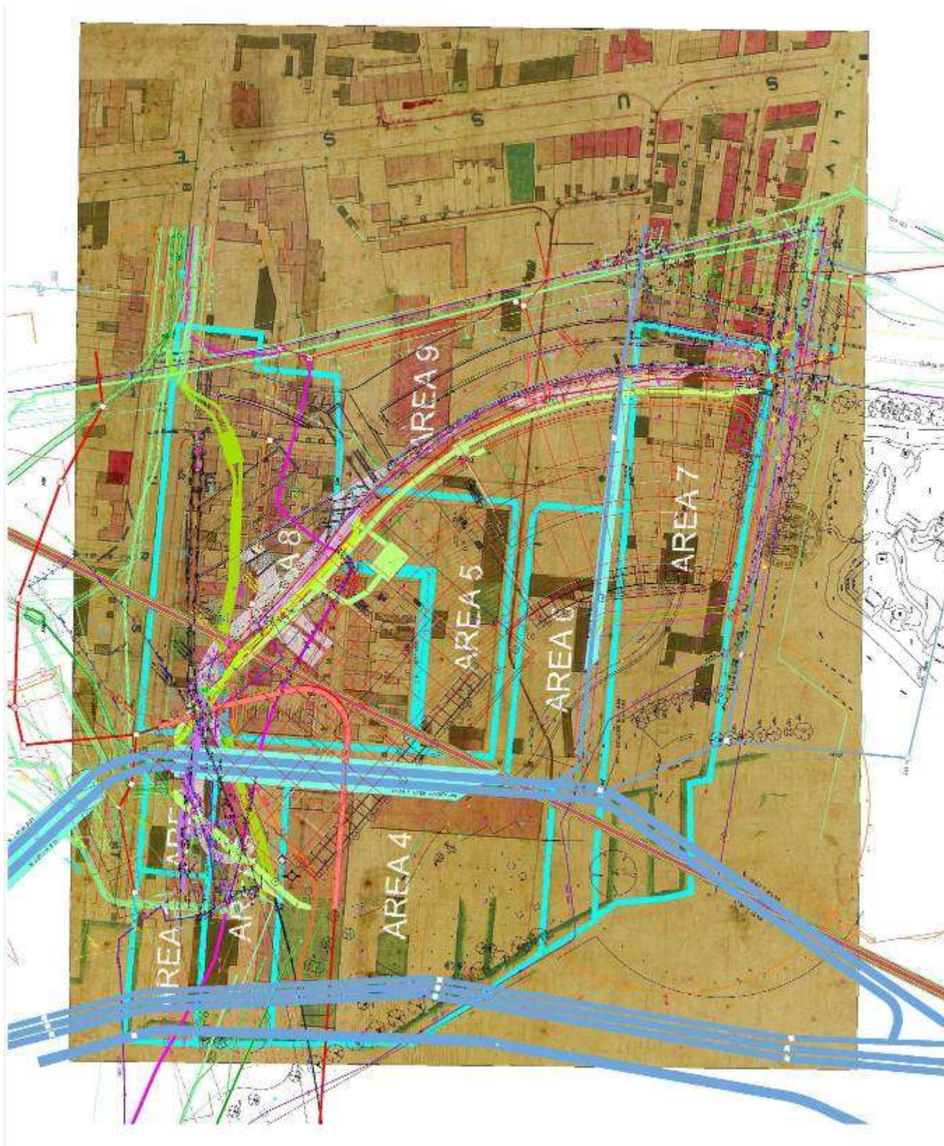
Figure 3.3: Overlay of the Darling Quarter (Walk) Site with elements of the SICEEP public domain and existing stormwater culverts. This plan shows that archaeology from Area 7 extends into the public domain (beneath Tumbalong Park) area as well as part of Area 6. Area 6 includes the remains of Barker's Jetty. It also shows the impacts from major culverts (blue lines) running through this area. North is at the left. Rygates for Casey & Lowe 2008b.
