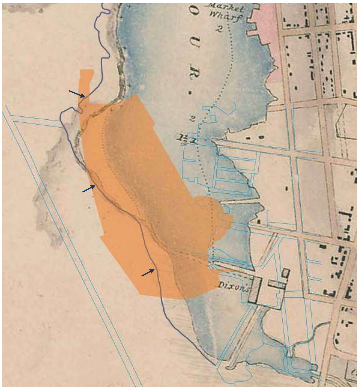
Figure 2.7: An 1828 plan showing the development of “Dixon’s” mill at Darling Harbour. Features include the pier extending into navigable water, and the wall retaining freshwater in the millpond and separating it from the harbour’s salt water. The dark blue line on the western foreshore (arrowed) illustrates the edge of the shoreline in 1854, from Woolcott & Clarke’s map. Therefore the area to the east of the dark blue line is probably mud flats. SR Item No: SZ467 SRNSW, accessed at acli.arts.usyd.edu.au .
