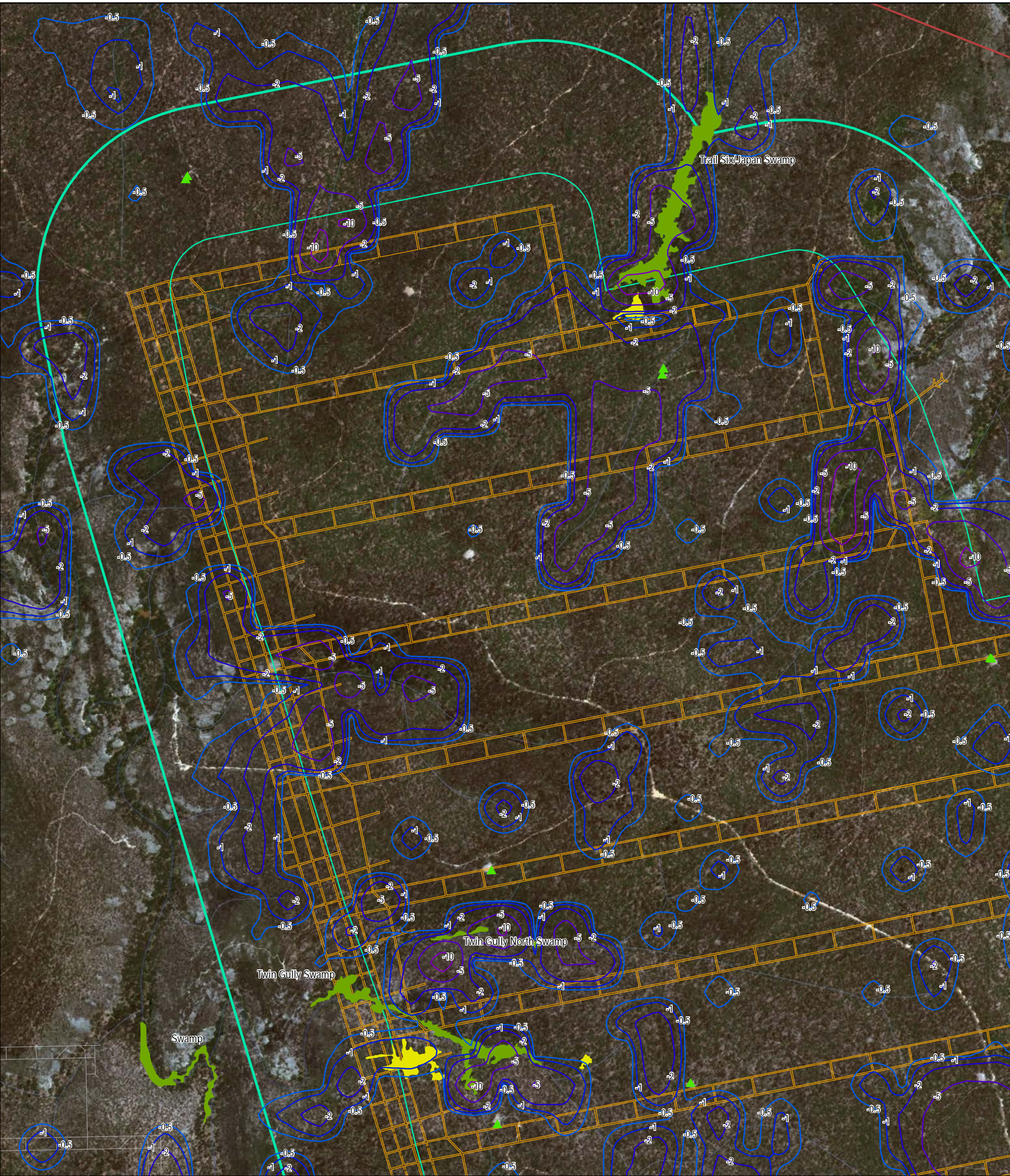
Figure 5.13: Predicted Drawdown at End of Mining – Twin Gully and Trail Six Swamps
