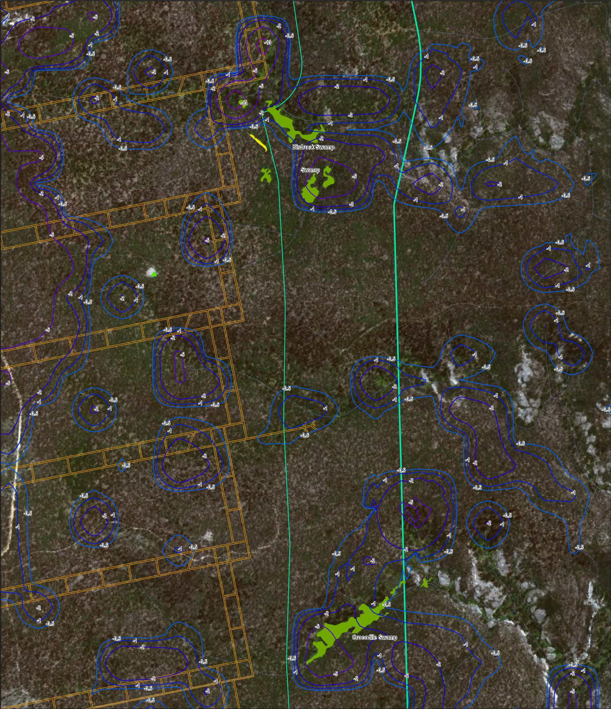
Figure 5.14: Predicted Drawdown at End of Mining – Birds Rock and Crocodile Swamps
