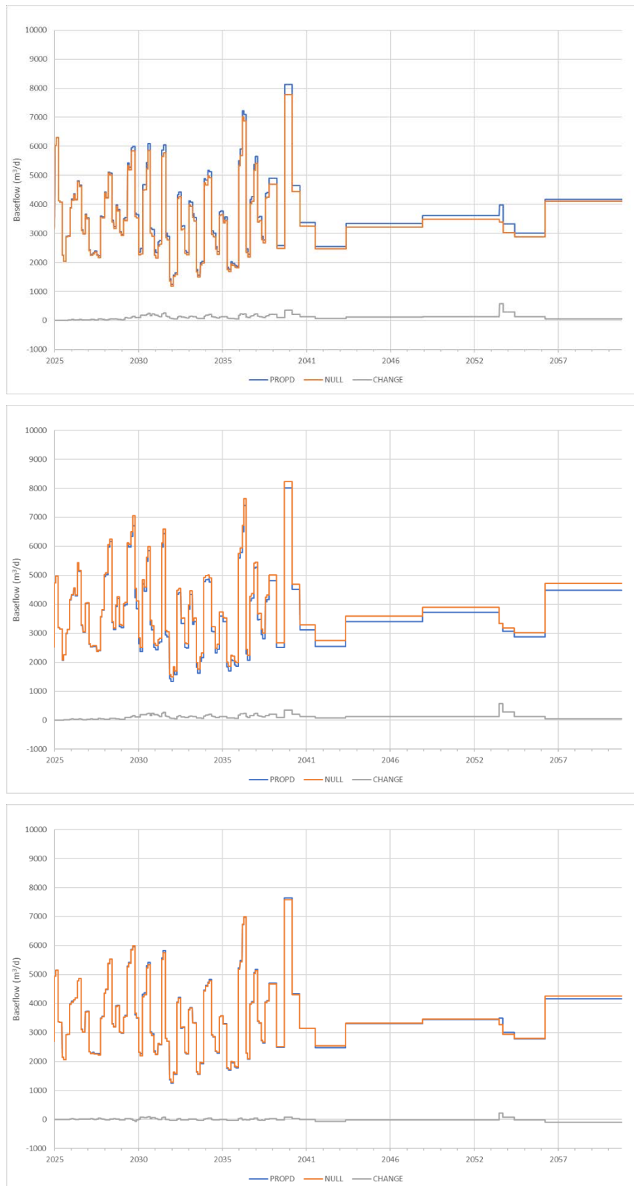
Figure A.3: Time-Series Model Output (CC02) – Carne Creek, East of LW1011 (Node NAT490a): Baseflow and Change in Baseflow (m 3 /d) (Upper is 10 th percentile; Middle is 90 th percentile; Bottom is SIM0)
