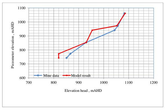
Figure B27 Comparison of observed and simulated piezometer elevation head profiles AP2PR (Date 01/01/2012)
