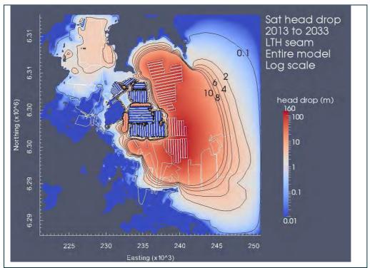
Figure 74 Drawdown in 2033 with respect to groundwater levels in January 2013 (entire model)
