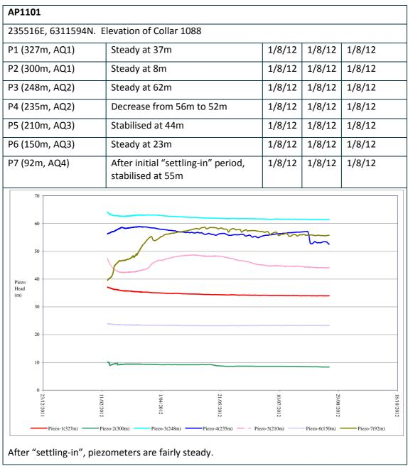
Figure A20 Description of piezometer hole AP1101
