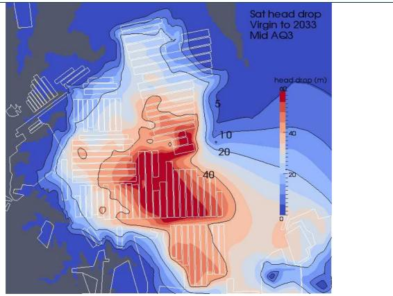
Figure D12 Distribution of drawdowns in AQ3 in 2033 with respect to pre-mining groundwater condition
