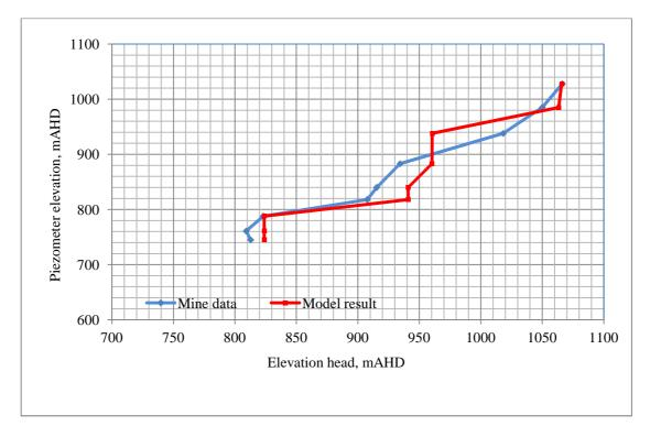
Figure B28 Comparison of observed and simulated piezometer elevation head profiles AP10PR (Date 01/01/2012)
