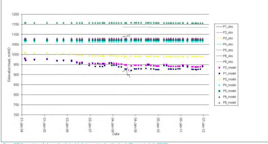
Figure B20 Comparison of observed and simulated piezometer elevation heads (Piezometer hole SPR49)
