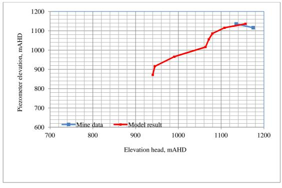
Figure B48 Comparison of observed and simulated piezometer elevation head profiles SPR49 (Date 01/01/2012, Note Piezo 1 to 6 got damaged)
