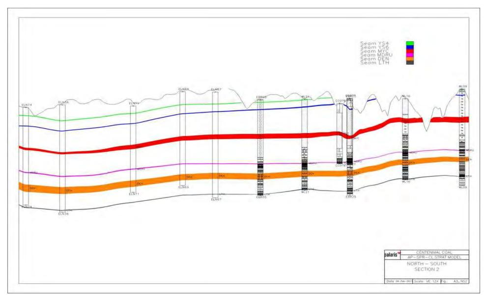
Figure 15 Geological cross-section NS2 showing Lithgow Seam (aqua), Denman Formation (grey), Katoomba Seam (pink), Mt York Claystone (red), YS6 (blue) and YS4 (Green) (detailed geological model; Palaris, 2013a)
