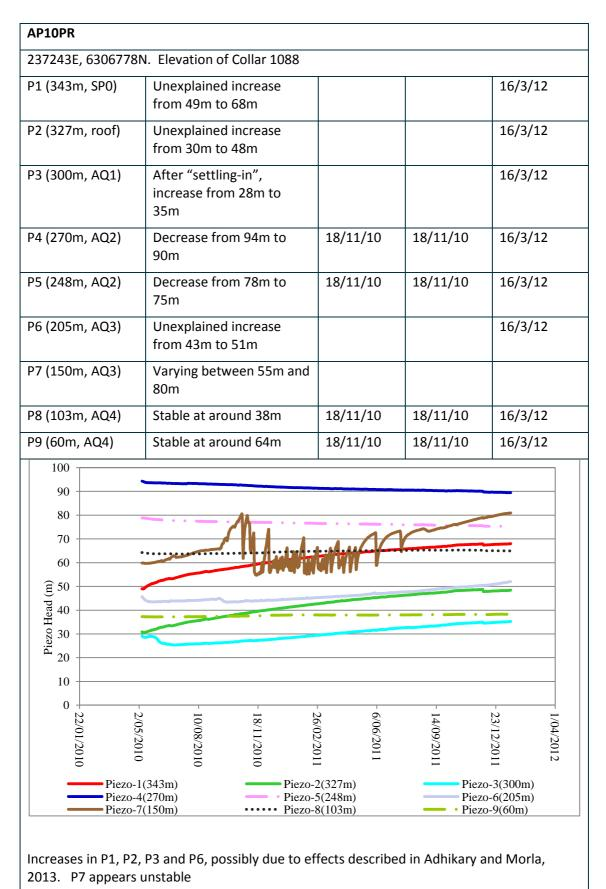
Figure A25 Description of piezometer hole AP10PR
