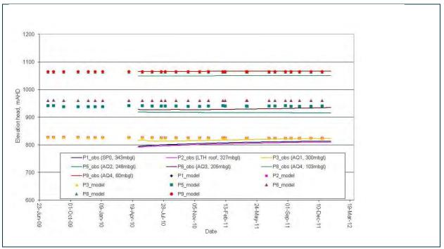
Figure 46 Comparison of observed and simulated piezometer elevation heads for AP10PR located in the chain pillar between APE-4 and APE-5 longwall panels away from the current mining activities, piezo depths range from 103mbgl to 343mbgl
