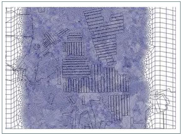
Figure 33 Closeup view of the fine mesh over the Springvale and Angus Place region
