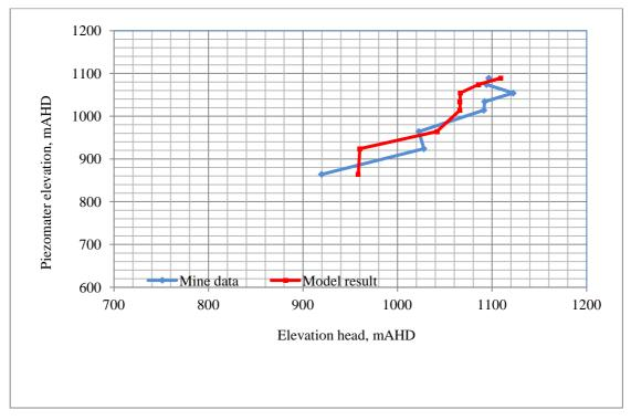
Figure B56 Comparison of observed and simulated piezometer elevation head profiles SPR67 (Date 12/01/2010)
