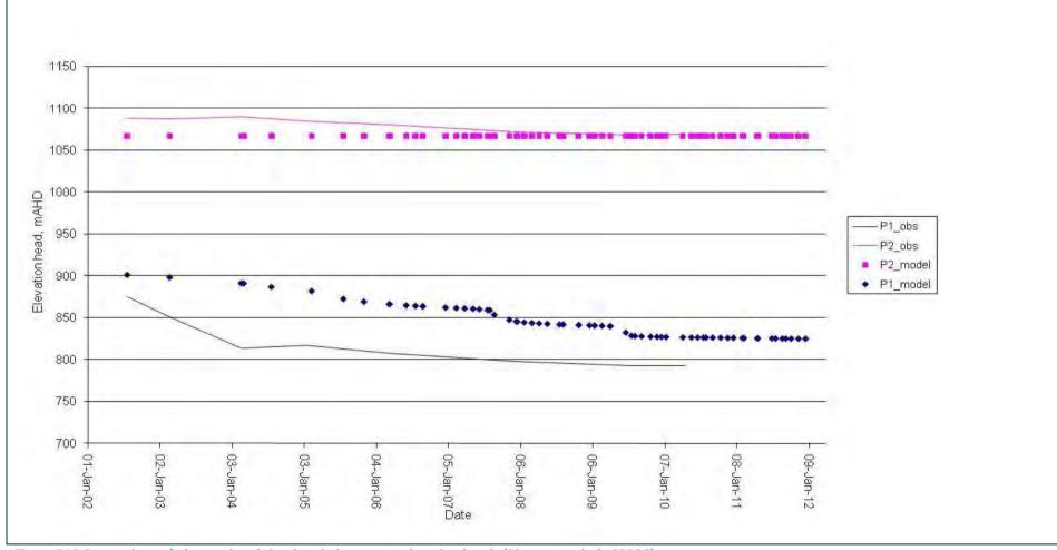
Figure B10 Comparison of observed and simulated piezometer elevation heads (Piezometer hole SPR26)
