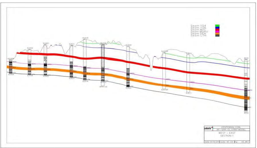
Figure 12 to Figure 15 present four stratigraphic cross-sections (marked in Figure 10) within the Angus Place and Springvale Colliery region. These cross-sections show that the aquicludes considered in the model are fairly continuous and consistent with the regional geological setting.
