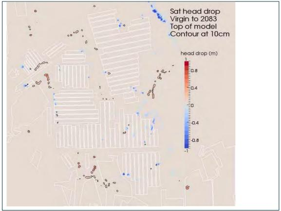
Figure 94 Distribution of saturated head drops at the ground surface in 2083 with respect to pre-mining groundwater condition.
