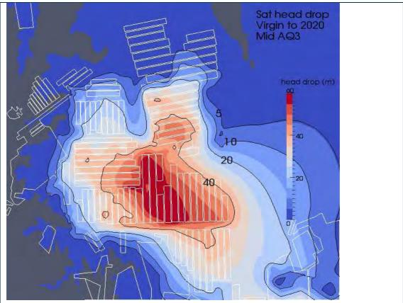
Figure D10 Distribution of drawdowns in AQ3 in 2020 with respect to pre-mining groundwater condition
