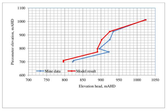
Figure B31 Comparison of observed and simulated piezometer elevation head profiles AP1102 (Date 01/04/2012)
