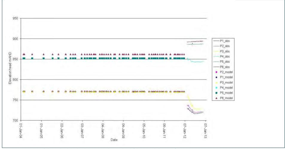
Figure B7 Comparison of observed and simulated piezometer elevation heads (Piezometer hole AP1106)
