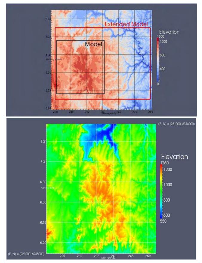
Figure 2 Model (black square) and Extended Model (red rectangle) extents, contoured by elevation of the topography
