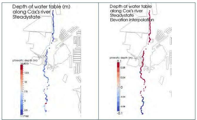
Figure 79 Depth of the watertable along Cox's river before any mining. Left picture: interpolation using the phreatic depth. Right picture: interpolation using the phreatic elevation. Notice that the depth is positive along most of Cox's river regardless of the interpolation used.
