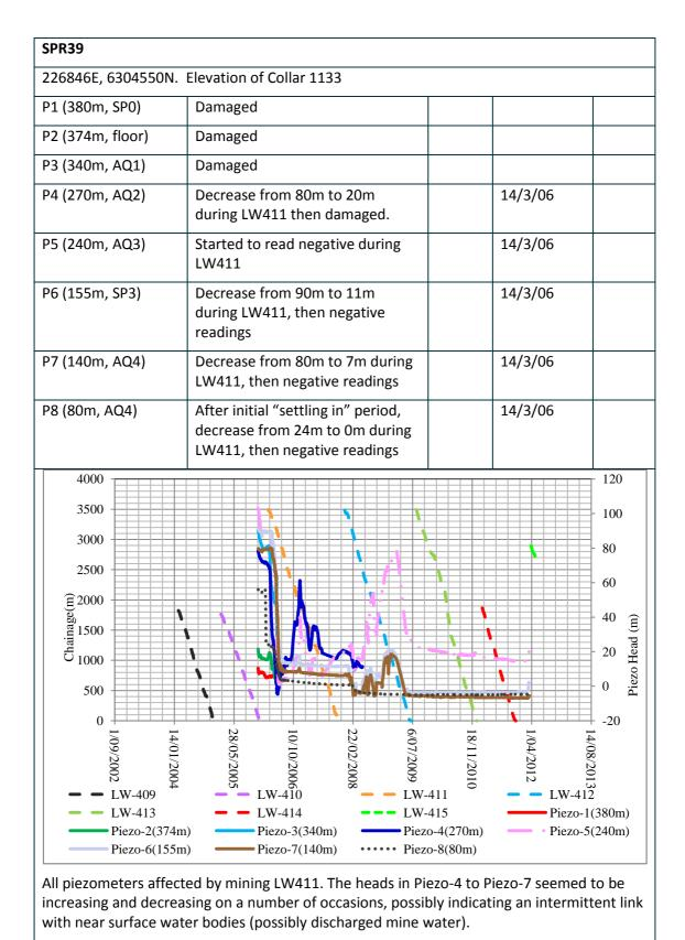
Figure A12 Description of piezometer hole SPR39
