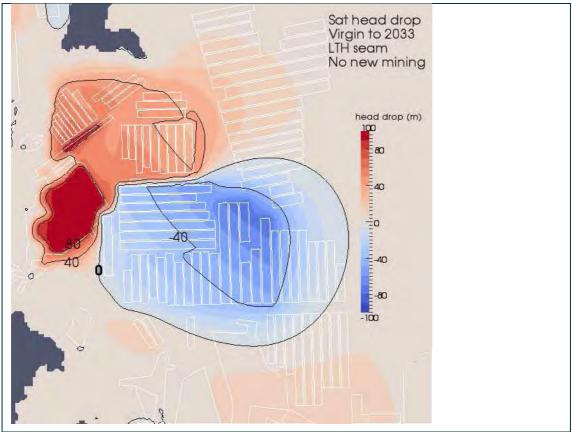
Figure D71 Distribution of head drops in the Lithgow seam at 2033 with respect to pre-mining conditions for the No New Mining scenario.
