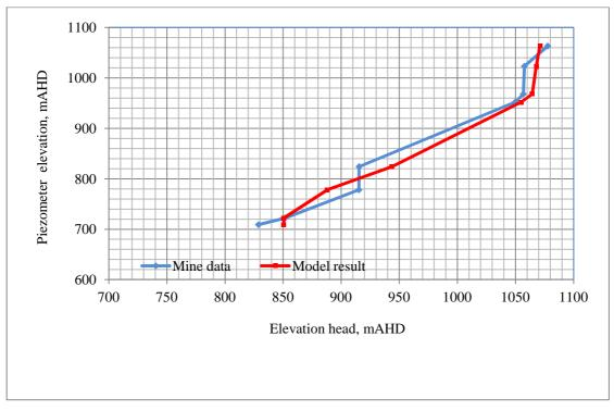
Figure B40 Comparison of observed and simulated piezometer elevation head profiles SPR36 (Date 12/01/2012)
