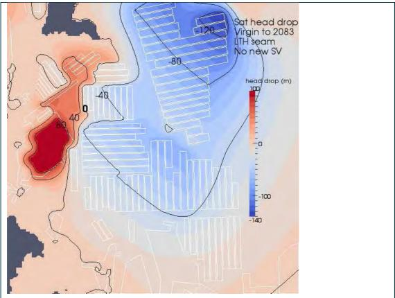
Figure D76 Distribution of head drops in the Lithgow seam at 2083 with respect to pre-mining conditions for the No New SV scenario
