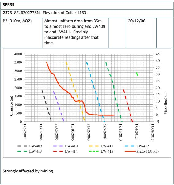
Figure A8 Description of piezometer hole SPR35
