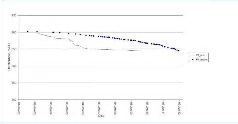
Figure B11 Comparison of observed and simulated piezometer elevation heads (Piezometer hole SPR29)
