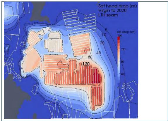
Figure D1 Distribution of drawdowns in the Lithgow Seam in 2020 with respect to pre-mining groundwater condition
