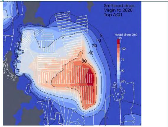
Figure D4 Distribution of drawdowns in AQ1 in 2020 with respect to pre-mining groundwater condition
