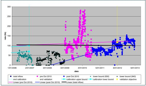
The flow rate at the end of validation should be 118 l/s which is also shown in Figure A30 by an yellow line and an yellow circle.
