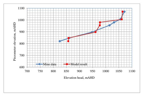
Figure B35 Comparison of observed and simulated piezometer elevation head profiles APB2 (Date 14/01/2012)
