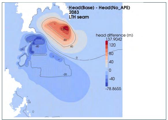
Figure D80 Head in the base model minus head in the No APE scenario at year 2083 for the Lithgow seam
