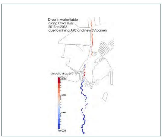
Figure 83 Drop in the phreatic surface along Cox's river between 2013 and 2033 due to mining APE and the new SV panels. A logarithmic scale has been used
