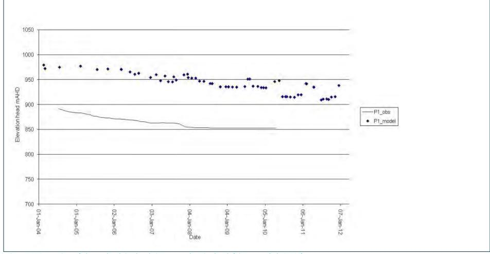
Figure B14 Comparison of observed and simulated piezometer elevation heads (Piezometer hole SPR35)
