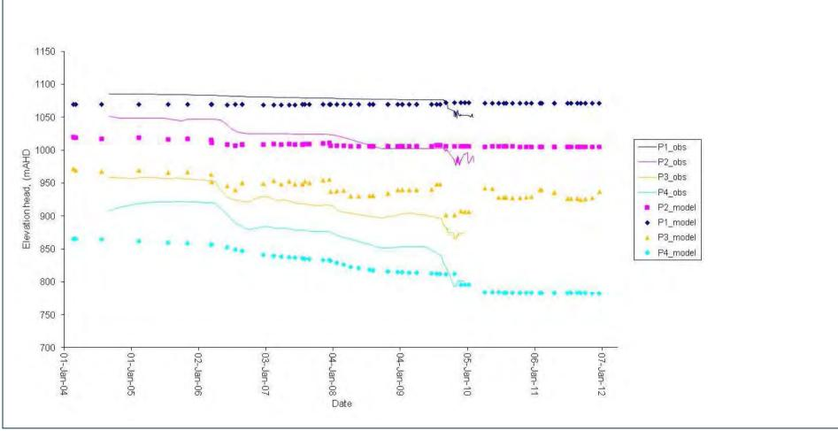
Figure B12 Comparison of observed and simulated piezometer elevation heads (Piezometer hole SPR33)
