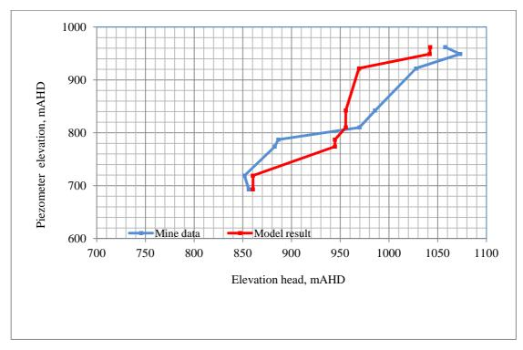
Figure B59 Comparison of observed and simulated piezometer elevation head profiles SPR1103 (Date 01/04/2012)
