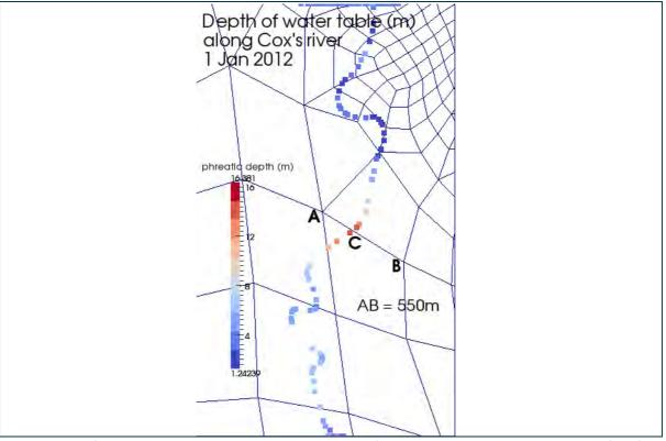
Figure 81 The finite element mesh is overlayed upon results from Figure 79. At the southern end of Cox's river, the interpolation is much less accurate since the element side-length is around 500m. By inspecting Figure 2, it is easy to imagine the interpolation from results at "A" and "B" to point "C" has significant error.
