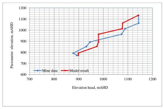
Figure B53 Comparison of observed and simulated piezometer elevation head profiles SPR64 (Date 12/10/2010)
