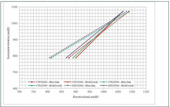
Figure 38 Comparison of observed and simulated head profile SPR26
