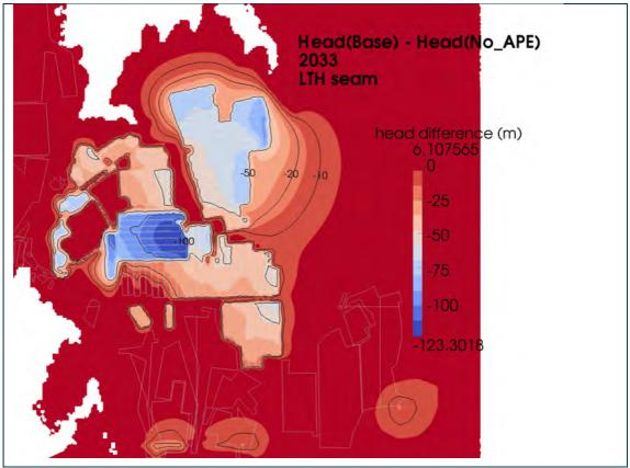
Figure D79 Head in the base model minus head in the No APE scenario at year 2033 for the Lithgow seam
