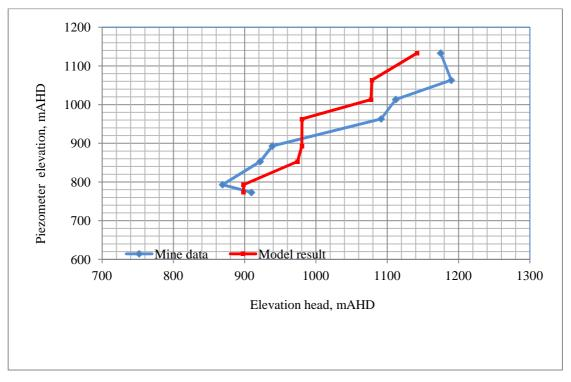
Figure B54 Comparison of observed and simulated piezometer elevation head profiles SPR64 (Date 01/01/2012)
