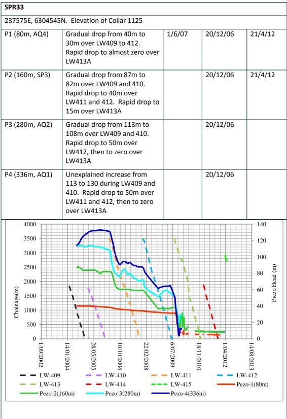
Strongly affected by mining. The initial increase in water head in Piezo-4 could be due to an issue with grouting or an effect described by Adhikary and Morla, 2013.
