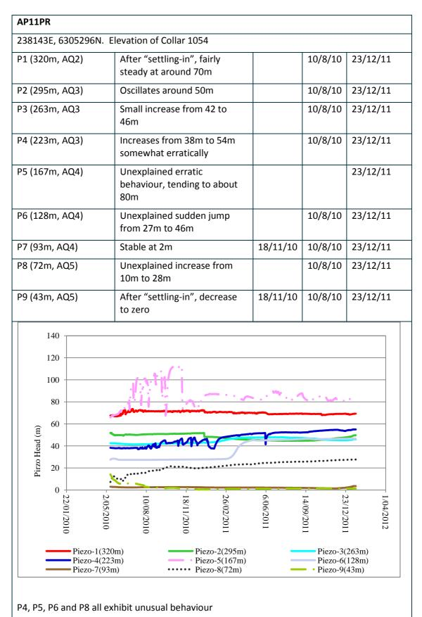
Figure A26 Description of piezometer hole AP11PR
