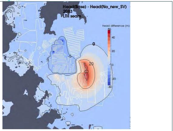
Figure D82 Head in the base model minus head in the No New SV scenario at year 2083 for the Lithgow seam
