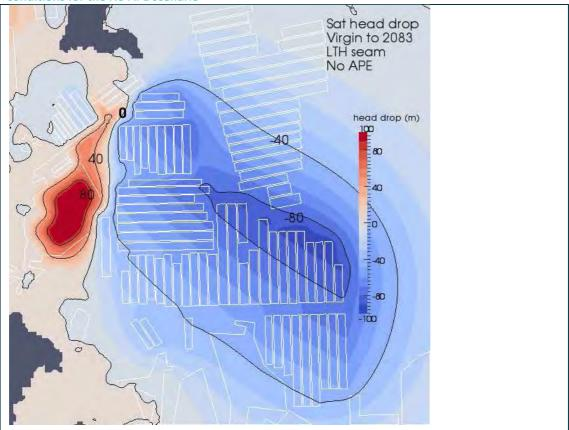
Figure D74 Distribution of head drops in the Lithgow seam at 2083 with respect to pre-mining conditions for the No APE scenario
