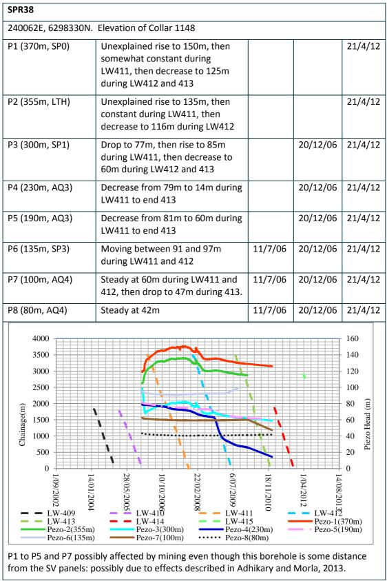
Figure A11 Description of piezometer hole SPR38
