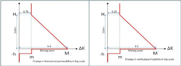
Figure 35 Calibrated ramp function representing change in permeability (log scale)
