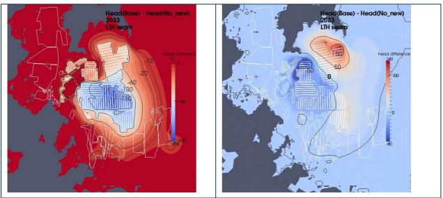
Figure 88. In the Lithgow seam at times 2033 (left) and 2083 (right). Contoured is the head of the base model minus the head of the "No New" scenario.
