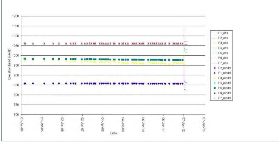
Figure B9 Comparison of observed and simulated piezometer elevation heads (Piezometer hole APB2)
