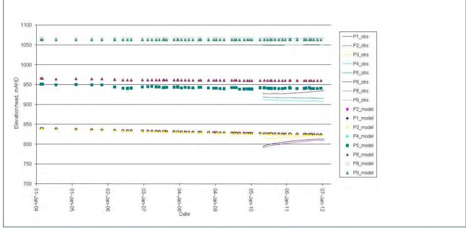
Figure B2 Comparison of observed and simulated piezometer elevation heads (Piezometer hole AP10PR)
