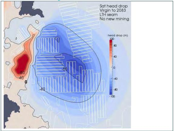
Figure D72 Distribution of head drops in the Lithgow seam at 2083 with respect to pre-mining conditions for the No New Mining scenario.
