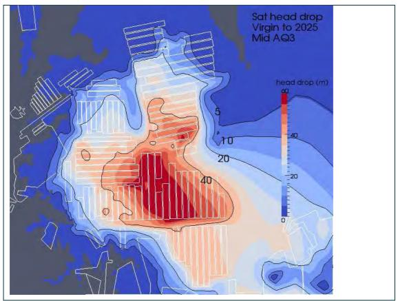
Figure D11 Distribution of drawdowns in AQ3 in 2025 with respect to pre-mining groundwater condition
