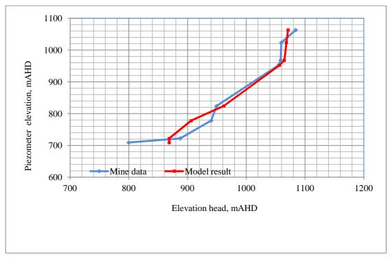
Figure B39 Comparison of observed and simulated piezometer elevation head profiles SPR36 (Date 12/03/2006)
