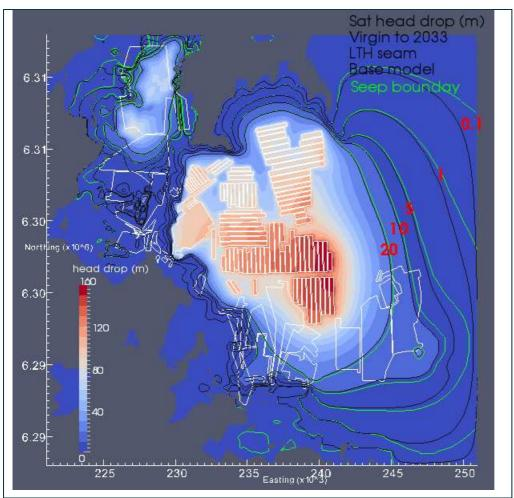
Figure 75 Drawdown in 2033 with respect to pre-mining groundwater condition (entire model)
