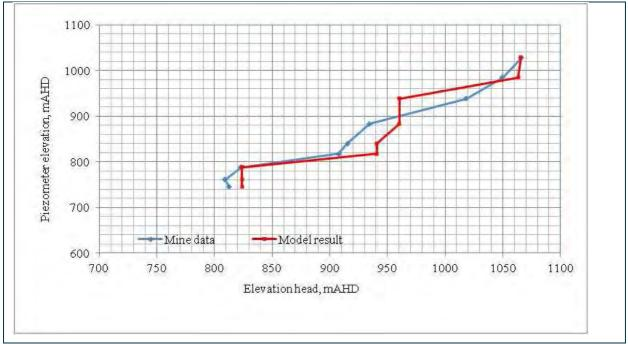
Figure 47 Comparison of observed and simulated piezometer elevation head profiles AP10PR (Date 01/01/2012)
