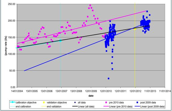
The flow rate at the end of validation should be 177 l/s which is also shown in Figure A29 by an yellow line and an yellow circle.
