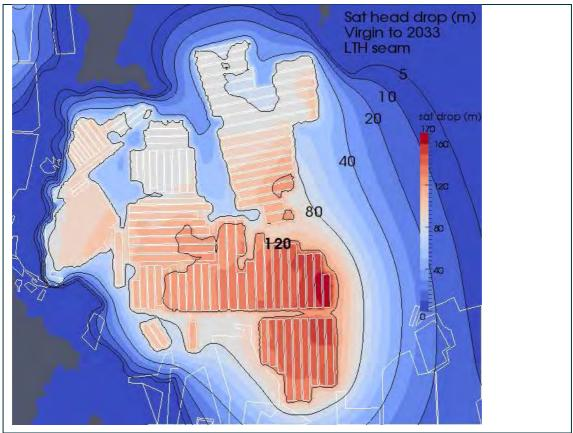
Figure D3 Distribution of drawdowns in the Lithgow Seam in 2033 with respect to pre-mining groundwater condition
