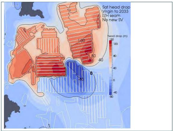
Figure D75 Distribution of head drops in the Lithgow seam at 2033 with respect to pre-mining conditions for the No New SV scenario
