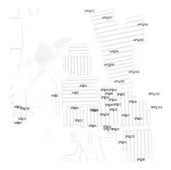
Figure A1 Position of boreholes containing piezometers used in this model
