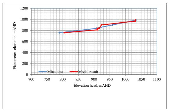
Figure B34 Comparison of observed and simulated piezometer elevation head profiles AP1107 (Date 01/01/2012)
