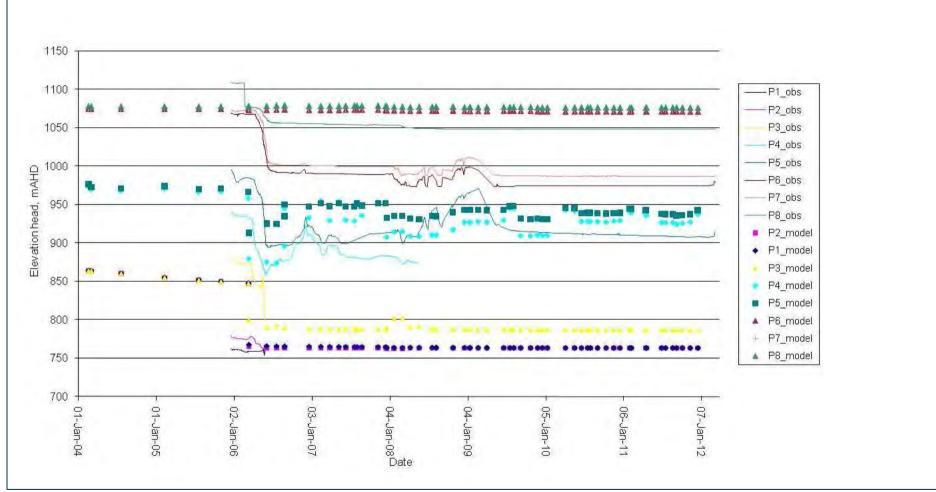
Figure B18 Comparison of observed and simulated piezometer elevation heads (Piezometer hole SPR39)
