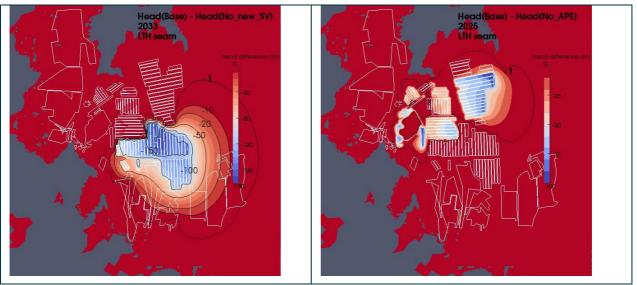
Figure 87 In the Lithgow seam at year 2033 (left) and year (right): the head of the Base model minus the Head of the "No new SV" and "No New APE" models
