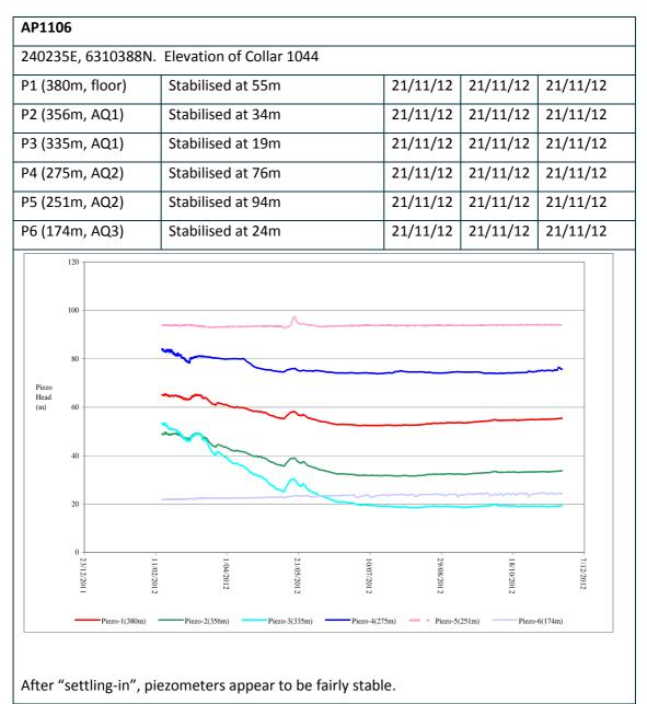
Figure A23 Description of piezometer hole AP1106
