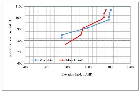
Figure B42 Comparison of observed and simulated piezometer elevation head profiles SPR37R (Date 13/03/2012)
