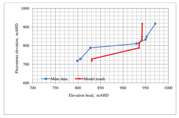
Figure B32 Comparison of observed and simulated piezometer elevation head profiles AP1104 (Date 01/01/2012)
