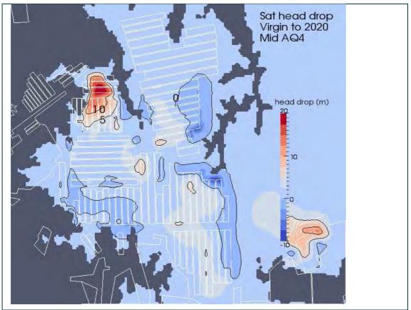
Figure D13 Distribution of drawdowns in AQ4 in 2020 with respect to pre-mining groundwater condition
