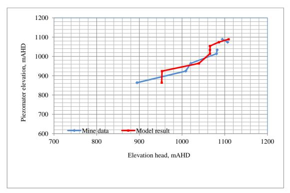
Figure B57 Comparison of observed and simulated piezometer elevation head profiles SPR67 (Date 01/01/2012)
