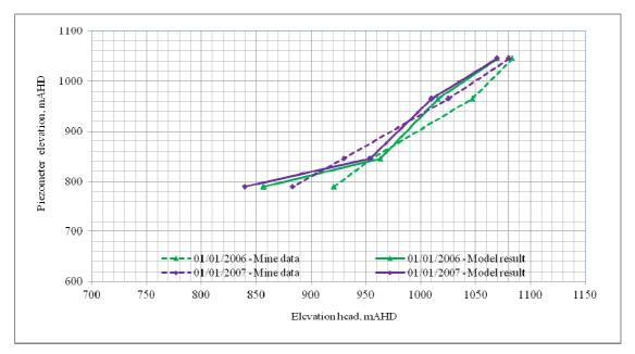
Figure B37 Comparison of observed and simulated piezometer elevation head profiles SPR33 (Date 1/01/2006)
