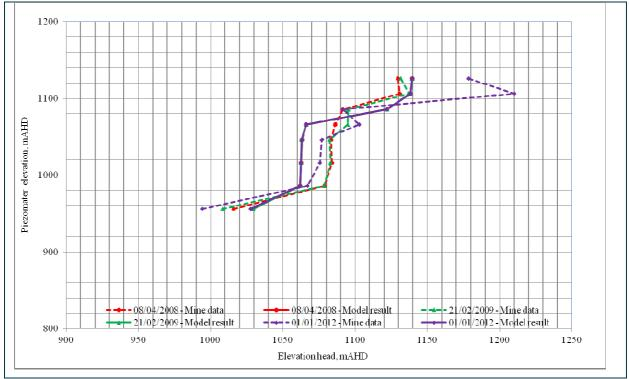
Figure 48 Comparison of observed and simulated piezometer elevation head profiles SPR50
