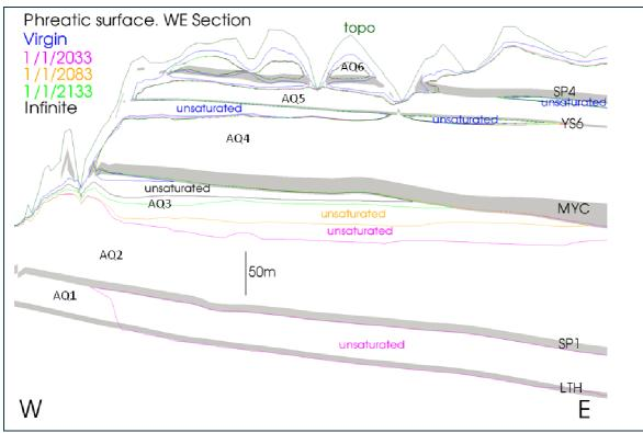
Figure 78 Phreatic surface before mining (blue lines), after mining (pink lines), 50 years after mining (yellow lines), 100 years after mining (green lines) and steady-state after mining (black lines) along E-W section
