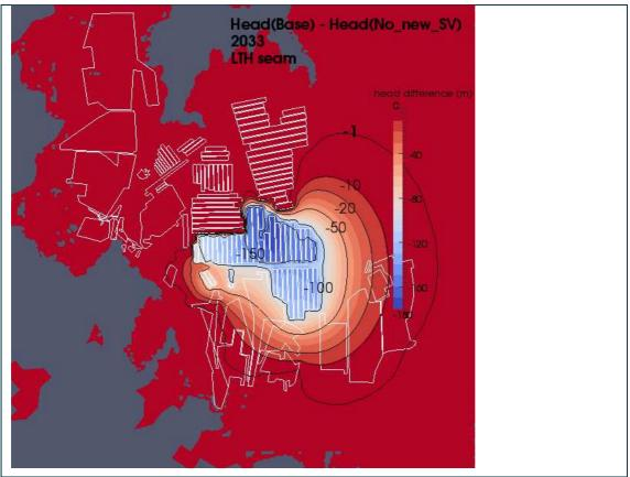
Figure D81 Head in the base model minus head in the No New SV scenario at year 2033 for the Lithgow seam
