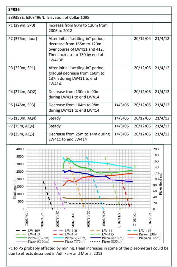
**Figure A9 Description of piezometer hole SPR36**
