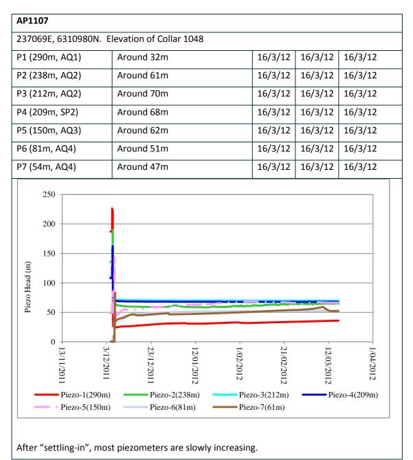
Figure A24 Description of piezometer hole AP1107
