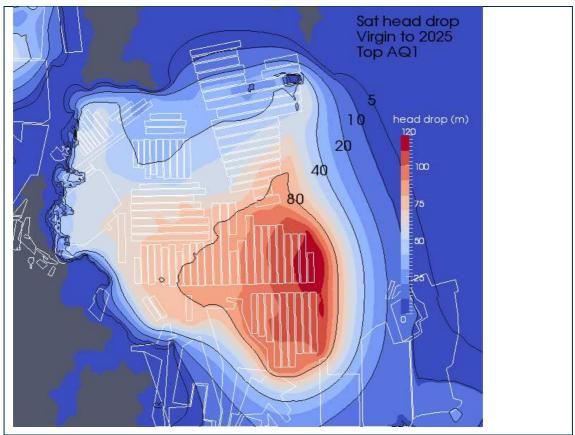
Figure D5 Distribution of drawdowns in AQ1 in 2025 with respect to pre-mining groundwater condition
