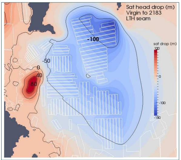
Figure 93 Distribution of head drops in the Lithgow Seam at 2183 with respect to pre-mining groundwater condition
