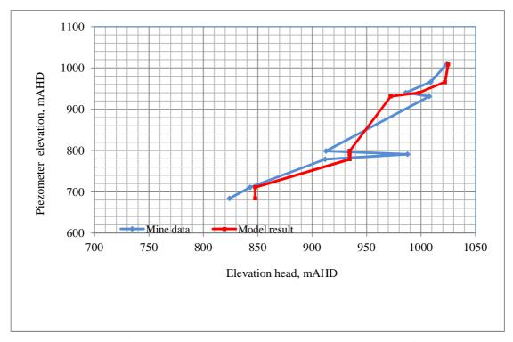
Figure B58 Comparison of observed and simulated piezometer elevation head profiles SPR1102 (Date 01/04/2012)
