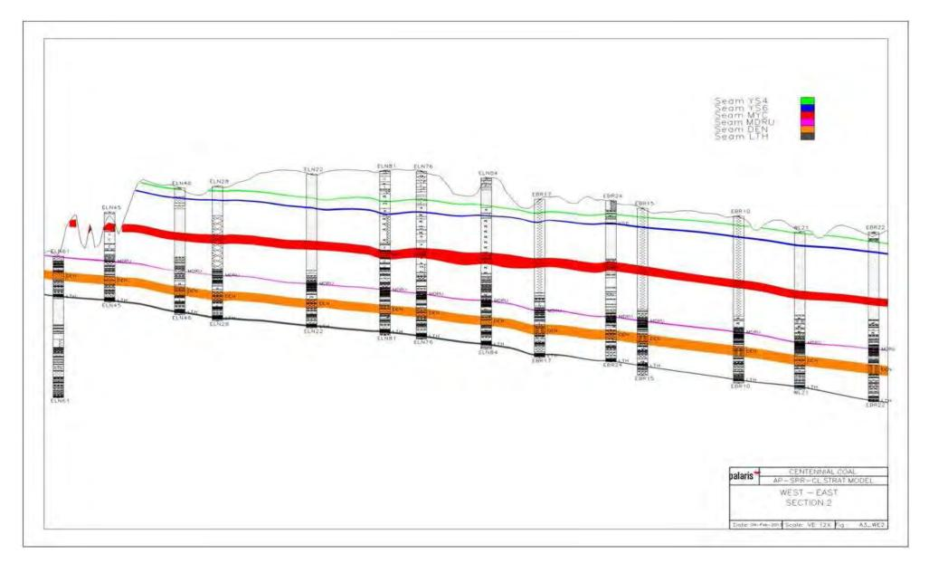
Figure 13 Geological cross-section WE2 showing Lithgow Seam (aqua), Denman Formation (grey), Katoomba Seam (pink), Mt York Claystone (red), YS6 (blue) and YS4 (Green) (detailed geological model; Palaris, 2013a)
