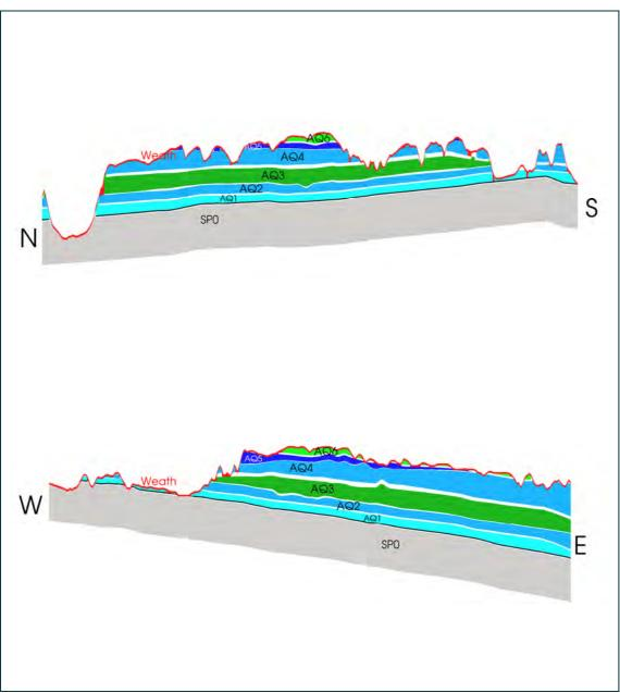
Figure 19 Two vertical cross-sections through the centre of the model. Colours indicate the material, and the topmost "Weath" layer is shown in red. The vertical exaggeration is 10
