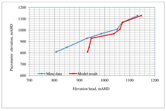
Figure B52 Comparison of observed and simulated piezometer elevation head profiles SPR51 (Date 01/01/2012)
