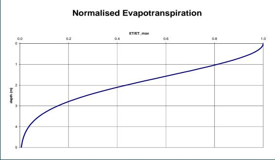
Figure 21 ET/Emax as a function of depth used in the model
