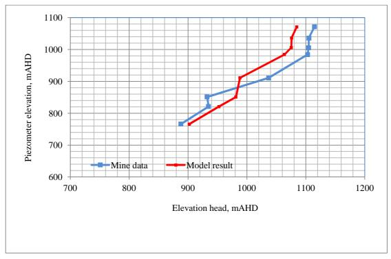
Figure B41 Comparison of observed and simulated piezometer elevation head profiles SPR37R (Date 12/03/2006)
