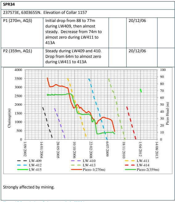
Figure A7 Description of piezometer hole SPR34
