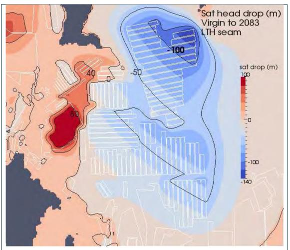
Figure 92 Distribution of head drops in the Lithgow Seam at 2083 with respect to pre-mining groundwater condition
