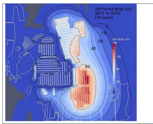
Figure 72 Distribution of drawdown in the Lithgow Seam in January 2033 with respect to groundwater levels in January 2013
