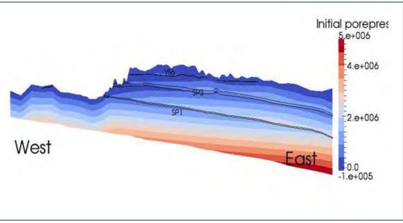
The porepressures and saturations thus achieved are interpolated onto the 'Model (mini-regional scale model)' yielding the distribution depicted in Figure 25
