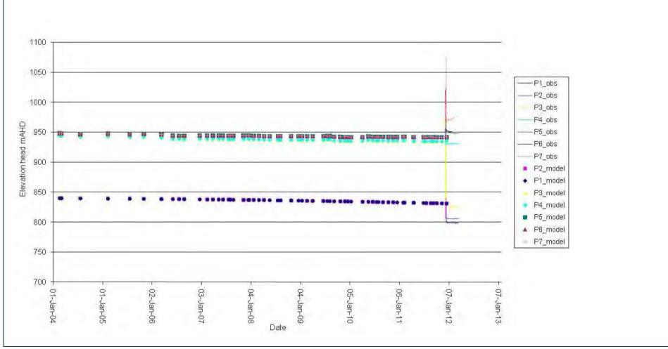
Figure B6 Comparison of observed and simulated piezometer elevation heads (Piezometer hole AP1104)
