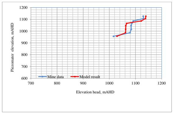
Figure B49 Comparison of observed and simulated piezometer elevation head profiles SPR50 (Date 08/04/2008)
