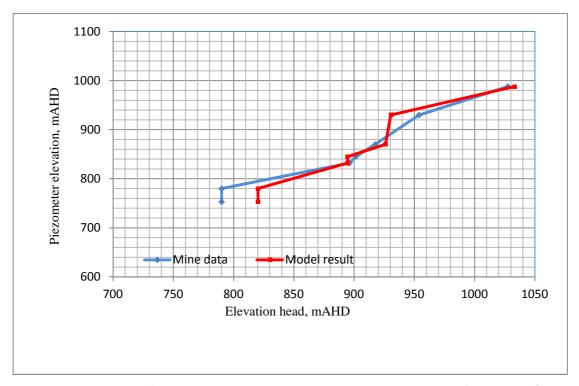
Figure B30 Comparison of observed and simulated piezometer elevation head profiles AP1101 (Date 01/04/2012)
