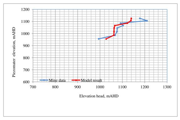
Figure B50 Comparison of observed and simulated piezometer elevation head profiles SPR50 (Date 01/01/2012)
