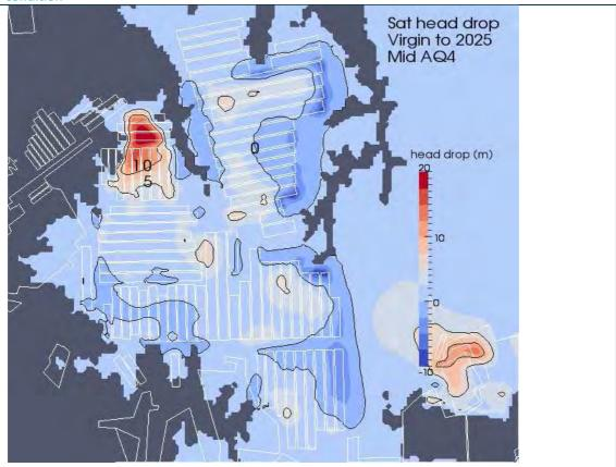
Figure D14 Distribution of drawdowns in AQ4 in 2025 with respect to pre-mining groundwater condition
