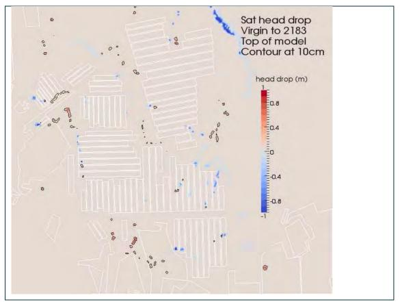
Figure 95 Distribution of saturated head drops at the ground surface in 2183 with respect to pre-mining groundwater condition
