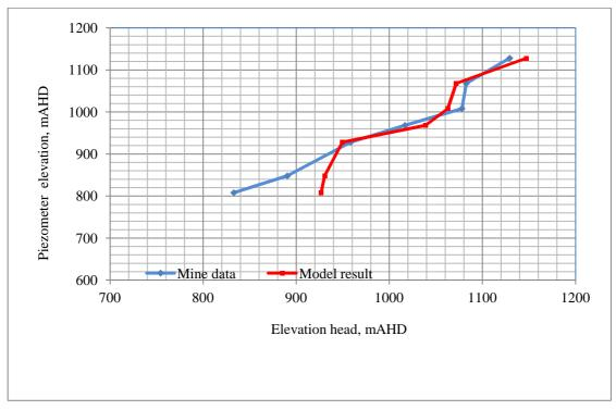
Figure B51 Comparison of observed and simulated piezometer elevation head profiles SPR51 (Date 20/01/2010)
