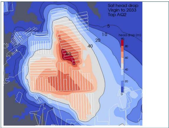
Figure D9 Distribution of drawdowns in AQ2 in 2033 with respect to pre-mining groundwater condition
