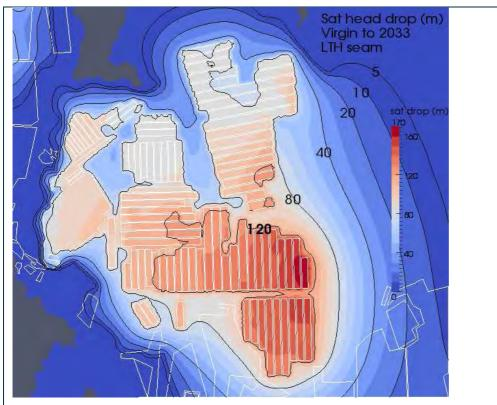
Figure 71 Distribution of drawdown in the Lithgow Seam in January 2033 with respect to pre-mining groundwater condition
