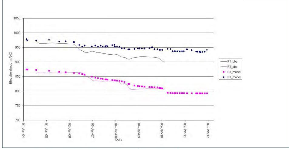
Figure B13 Comparison of observed and simulated piezometer elevation heads (Piezometer hole SPR34)
