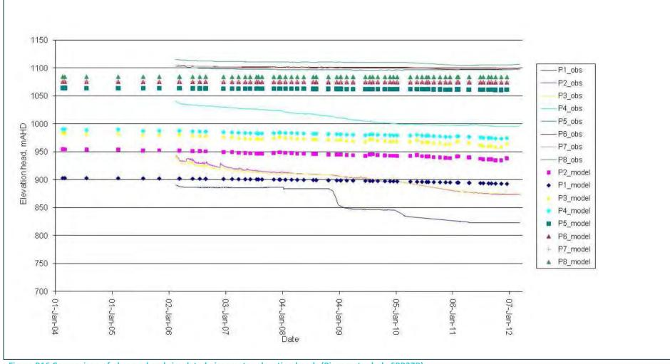
Figure B16 Comparison of observed and simulated piezometer elevation heads (Piezometer hole SPR37R)
