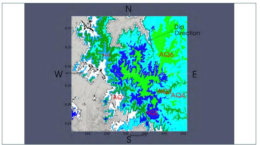
Figure 18 Surface geology generated within the model, with the weathered layer stripped away. The aquifers are coloured with different shades of blue and green, while the coal seam is black, and the basement (SPO) is grey. The layers are quite close to planar, and parallel, and their dip direction is 19 degrees north of east, as shown. The dip angle is 0.87 degrees, or 15m/1km. Finally, the position of two cross-sectional slices – WE and NS – is shown
