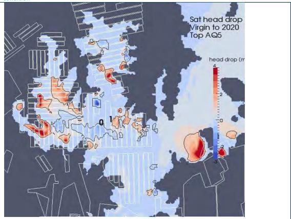
Figure D16 Distribution of drawdowns in AQ5 in 2020 with respect to pre-mining groundwater condition
