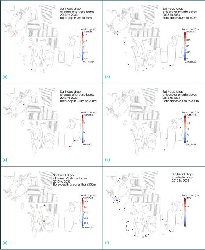
Figure 84 Head drops in private bores due to mining of the proposed APE and SV longwalls (Base case)
