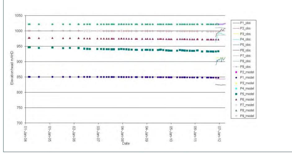
Figure B25 Comparison of observed and simulated piezometer elevation heads (Piezometer hole SPR1102)
