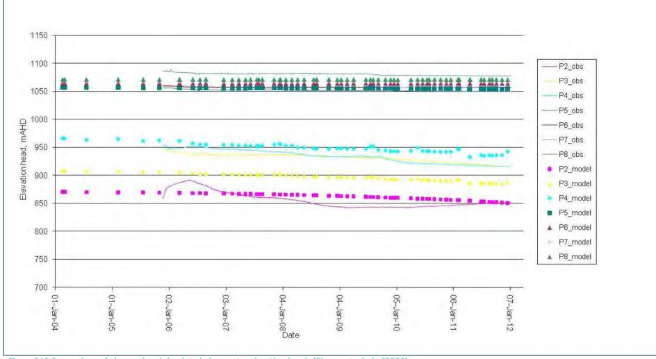
Figure B15 Comparison of observed and simulated piezometer elevation heads (Piezometer hole SPR36)
