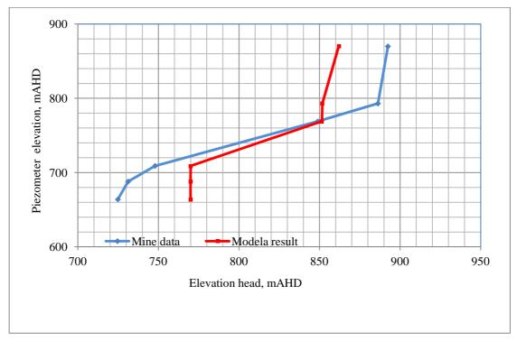
Figure B33 Comparison of observed and simulated piezometer elevation head profiles AP1106 (Date 01/04/2012)
