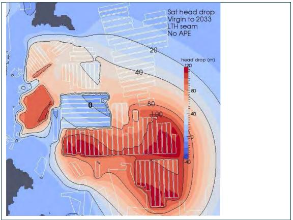
Figure D73 Distribution of head drops in the Lithgow seam at 2033 with respect to pre-mining conditions for the No APE scenario
