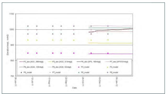
Figure 45 Comparison of observed and simulated piezometer elevation heads for SPR1102 located at the eastern margin of the proposed longwall panels at Springvale Colliery well away from the current mining activites, piezo depths range from 82mbgl to 380mbgl
