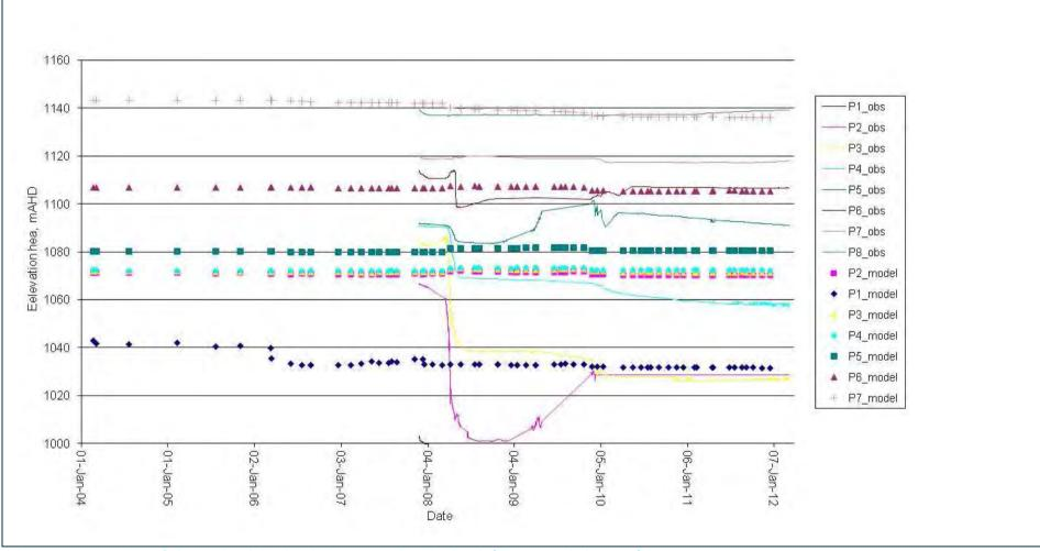
Figure B19 Comparison of observed and simulated piezometer elevation heads (Piezometer hole SPR48)
