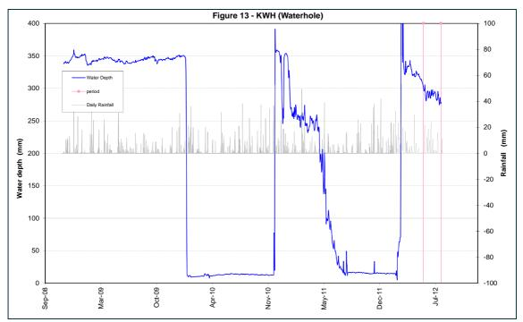
Figure A32 Water depth in the waterhole located close to the lower end of Kangaroo Swamp. As Angus Place LW950 passes under the waterhole in early 2010, its level drops.
