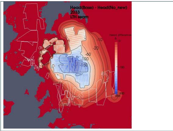
Figure D77 Head in the base model minus head in the No New scenario at year 2033 for the Lithgow seam
