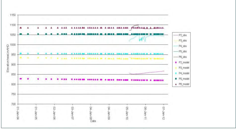
Figure B1 Comparison of observed and simulated piezometer elevation heads (Piezometer hole AP2PR)
