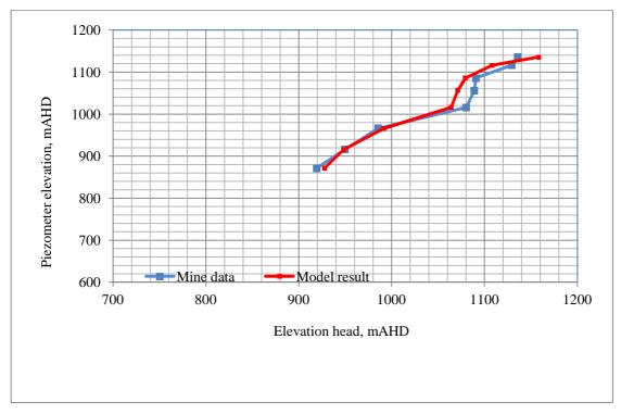
Figure B47 Comparison of observed and simulated piezometer elevation head profiles SPR49 (Date 20/07/2008)
