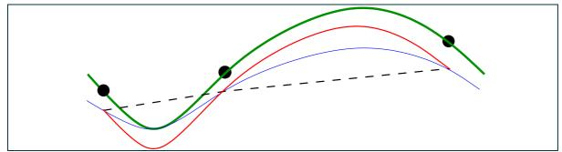
Figure 80 The phreatic surface (blue line) below the topography (green line)
