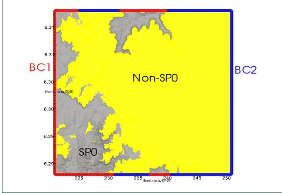
Figure 26 Two types of boundary conditions (BC1 or BC2) can be applied to the edges of the model. The colouring of the central region shows the model geology
