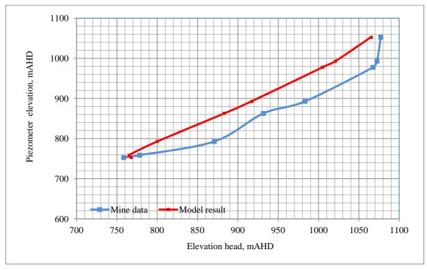
Figure B45 Comparison of observed and simulated piezometer elevation head profiles SPR39 (Date 01/01/2012)
