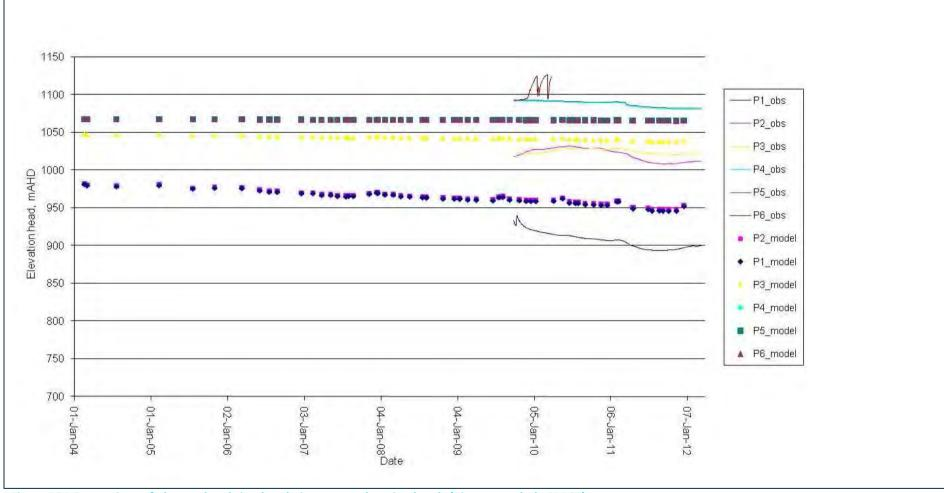
Figure B24 Comparison of observed and simulated piezometer elevation heads (Piezometer hole SPR67)
