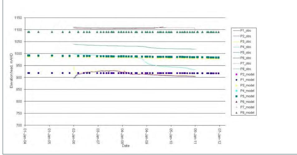
Figure B17 Comparison of observed and simulated piezometer elevation heads (Piezometer hole SPR38)
