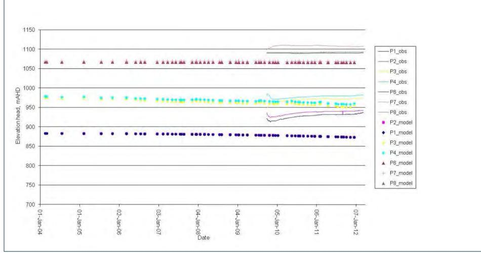
Figure B23 Comparison of observed and simulated piezometer elevation heads (Piezometer hole SPR66)
