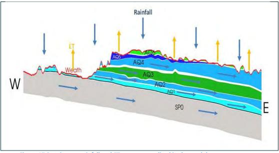
Figure 17 Stratigrapy, rainfall and ET as conceptualised in the model
