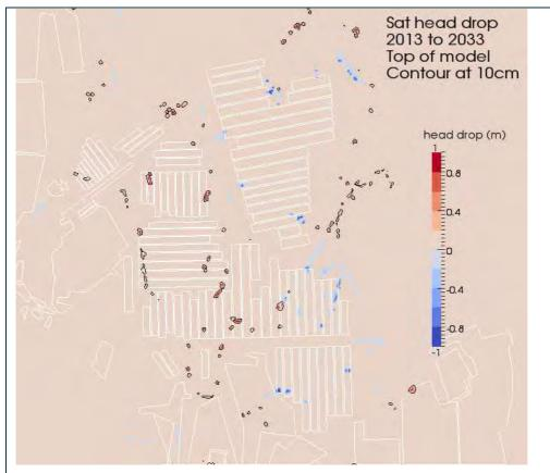
Figure 73 Distribution of head drops at the ground surface in January 2033 with respect to groundwater levels in January 2013
