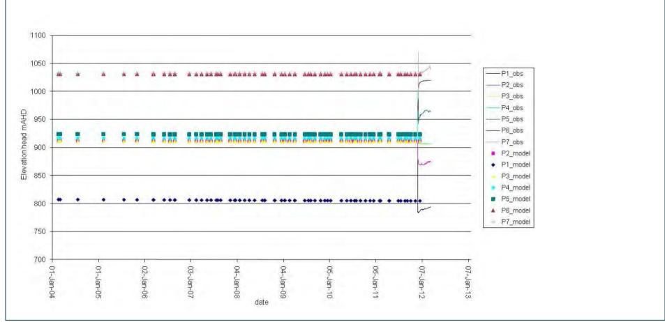
Figure B8 Comparison of observed and simulated piezometer elevation heads (Piezometer hole AP1107)
