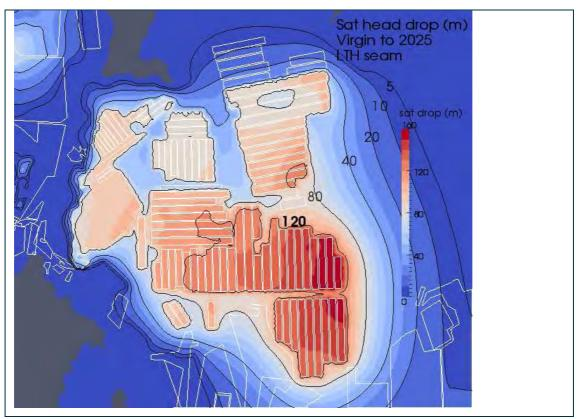
Figure D2 Distribution of drawdowns (m) in the Lithgow Seam in 2025 with respect to pre-mining groundwater condition
