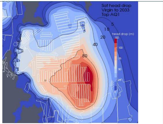
Figure D6 Distribution of drawdowns in AQ1 in 2033 with respect to pre-mining groundwater condition
