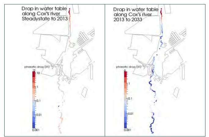
Figure 82 Drop in the phreatic surface along Cox's river between steady-state and 2013 (left), and 2013 and 2033 (right. A logarithmic scale has been used
