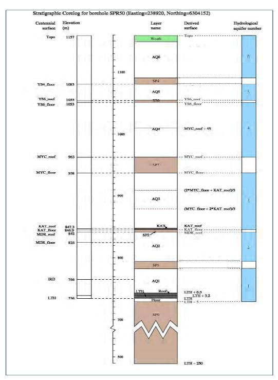
Figure 16 Model stratigraphy (right) and corelog showing elevation of geological surfaces supplied by Centennial Coal (left) at piezometer borehole SPR50 (238290E, 6304152N). Red dotted lines indicate subdivision of a single material layer into a number of finite element layers to improve vertical resolution
