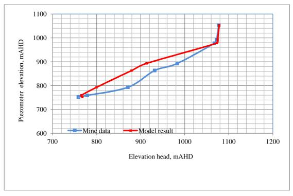
Figure B44 Comparison of observed and simulated piezometer elevation head profiles SPR39 (Date 24/03/2006)
