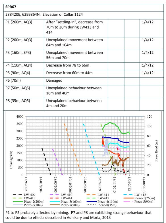
Figure A19 Description of piezometer hole SPR67
