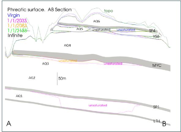
Figure 76 Phreatic surface before mining (blue lines), after mining (pink lines), 50 years after mining (yellow lines), 100 years after mining (green lines) and steady-state after mining (black lines) along A-B section
