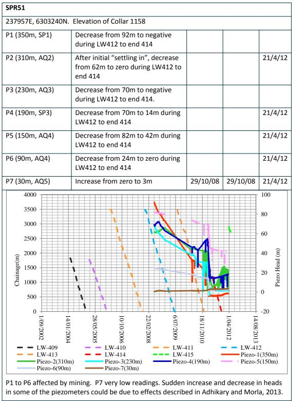
Figure A16 Description of piezometer hole SPR51
