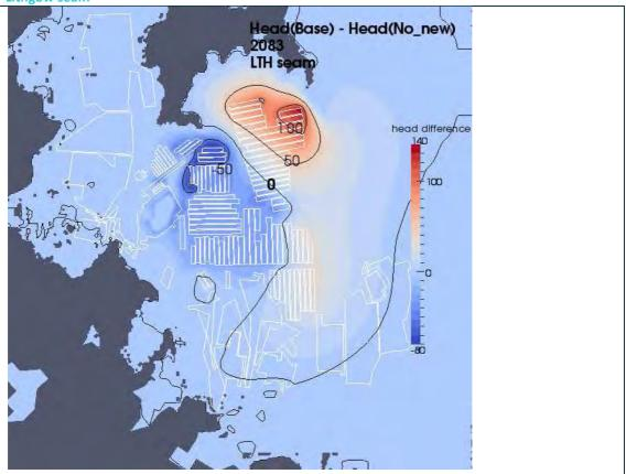
Figure D78 Head in the base model minus head in the No New scenario at year 2083 for the Lithgow seam
