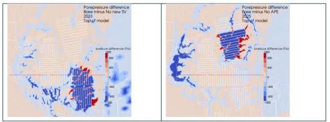
Figure 86 Porepressure change at the top of the model for two scenarios with respect to the Base case
