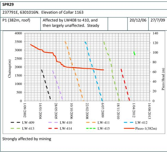
Figure A5 Description of piezometer hole SPR29
