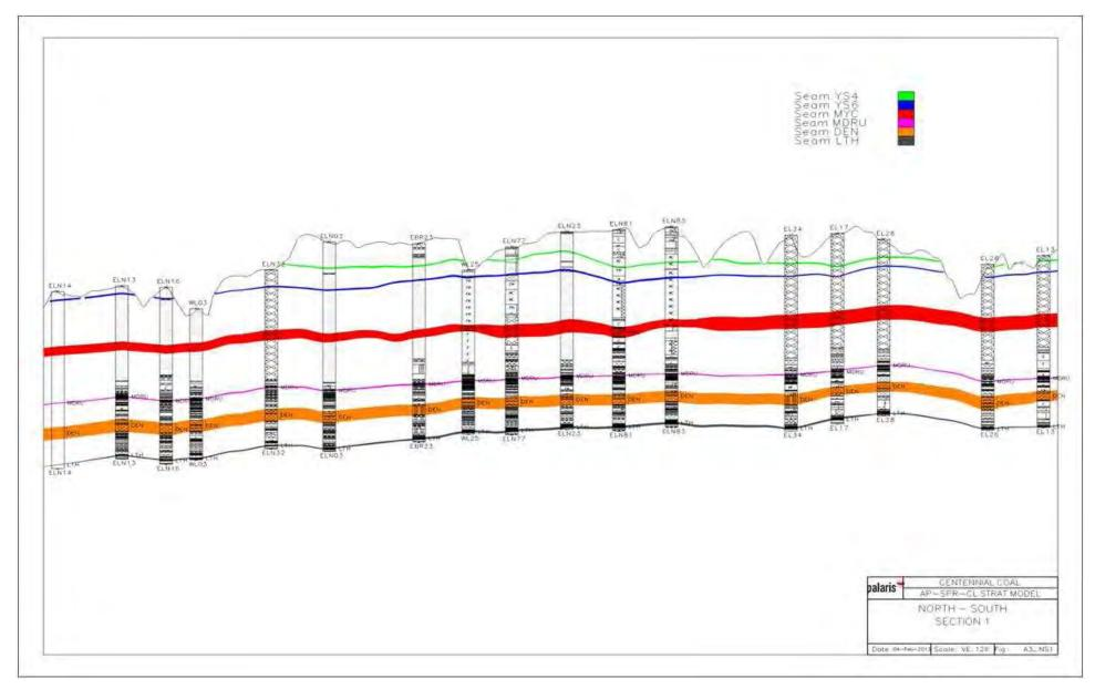
Figure 14 Geological cross-section NS1 showing Lithgow Seam (aqua), Denman Formation (grey), Katoomba Seam (pink), Mt York Claystone (red), YS6 (blue) and YS4 (Green) (detailed geological model; Palaris, 2013a)
