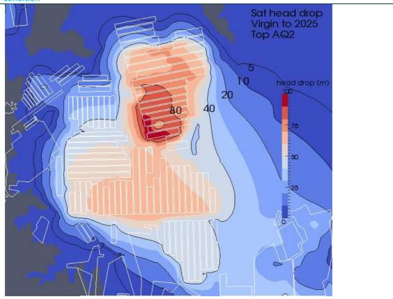
Figure D8 Distribution of drawdowns in AQ2 in 2025 with respect to pre-mining groundwater condition
