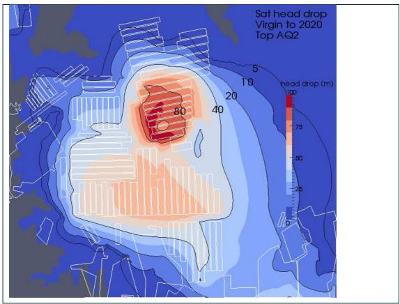
Figure D7 Distribution of drawdowns in AQ2 in 2020 with respect to pre-mining groundwater condition
