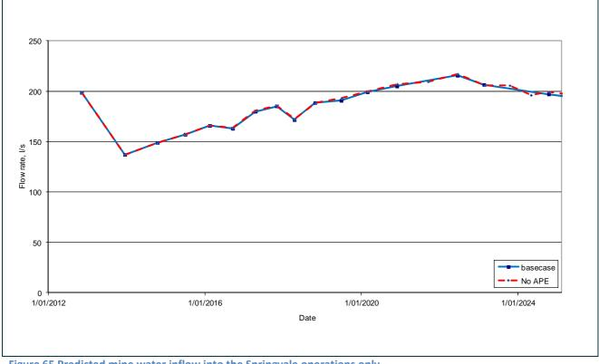
Figure 65 Predicted mine water inflow into the Springvale operations only
