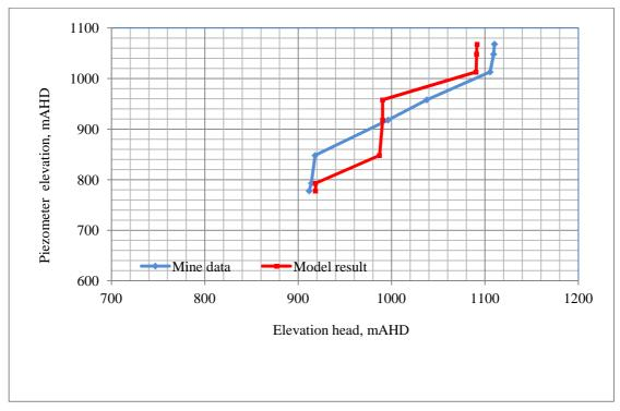
Figure B43 Comparison of observed and simulated piezometer elevation head profiles SPR38 (Date 12/03/2006)
