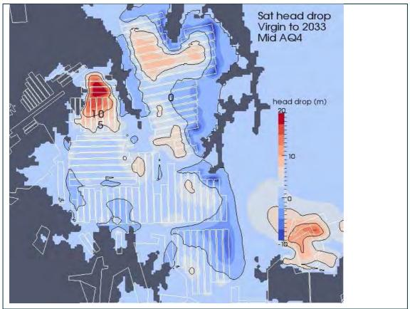
Figure D15 Distribution of drawdowns in AQ4 in 2033 with respect to pre-mining groundwater condition
