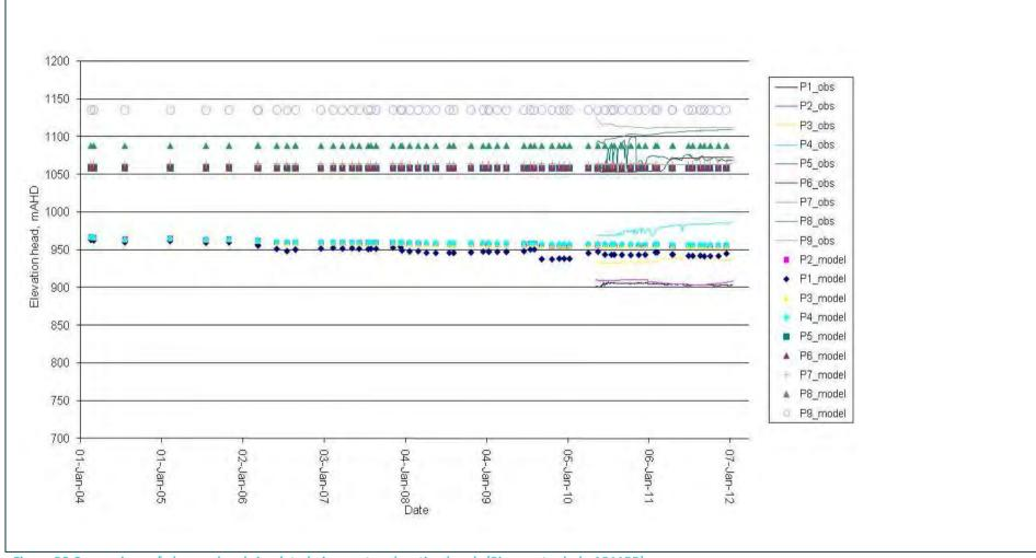
Figure B3 Comparison of observed and simulated piezometer elevation heads (Piezometer hole AP11PR)
