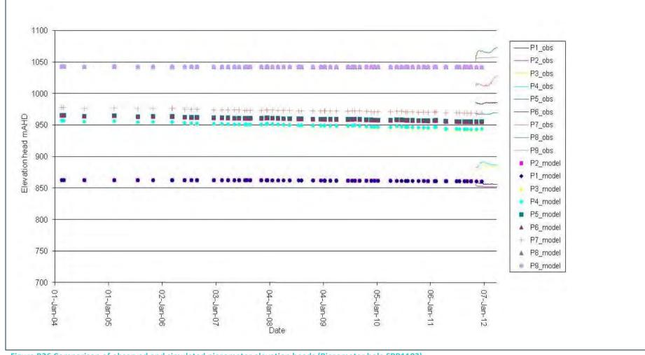
Figure B26 Comparison of observed and simulated piezometer elevation heads (Piezometer hole SPR1103)
