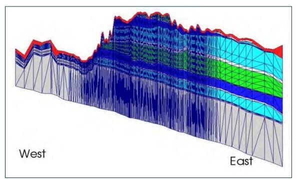
Figure 34 West-East vertical cross section through the centre of the model showing the vertical mesh. Coloured by material layer. This picture is similar to Figure 19, however here the vertical exaggeration is 20
