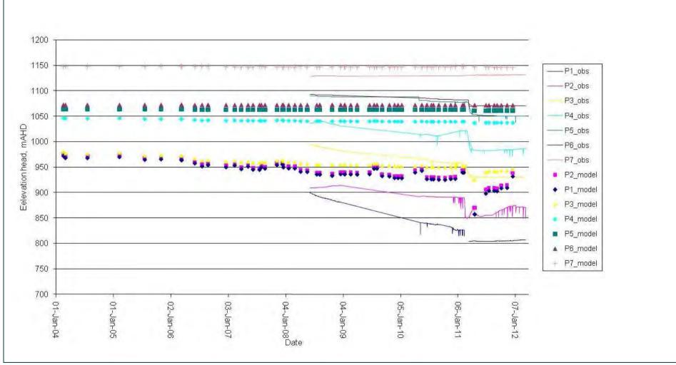
Figure B22 Comparison of observed and simulated piezometer elevation heads (Piezometer hole SPR51)
