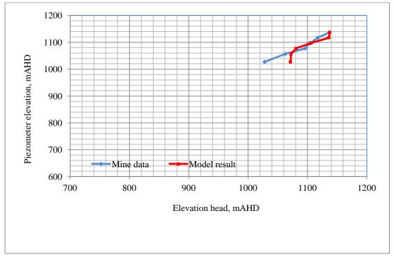
Figure B46 Comparison of observed and simulated piezometer elevation head profiles SPR48 (Date 01/01/2012)
