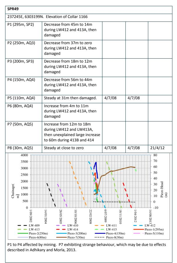
Figure A14 Description of piezometer hole SPR49
