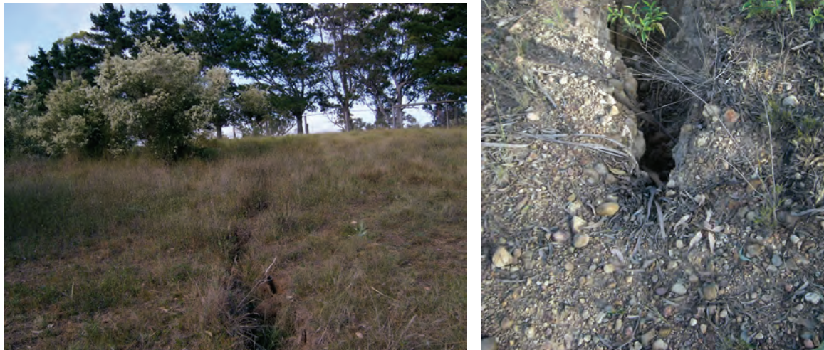
Fig. 5.17 Photographs of Typical Tension Cracks on Steep Slopes from the NSW Coalfields
