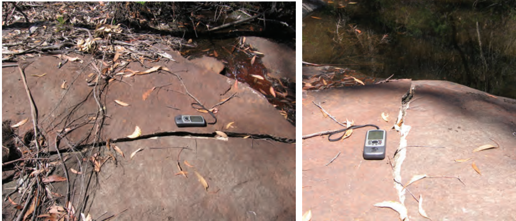
Fig. 4.6 Photographs of Fracturing along Kangaroo Creek due to Valley Closure above Angus Place LW920 (after Centennial)
