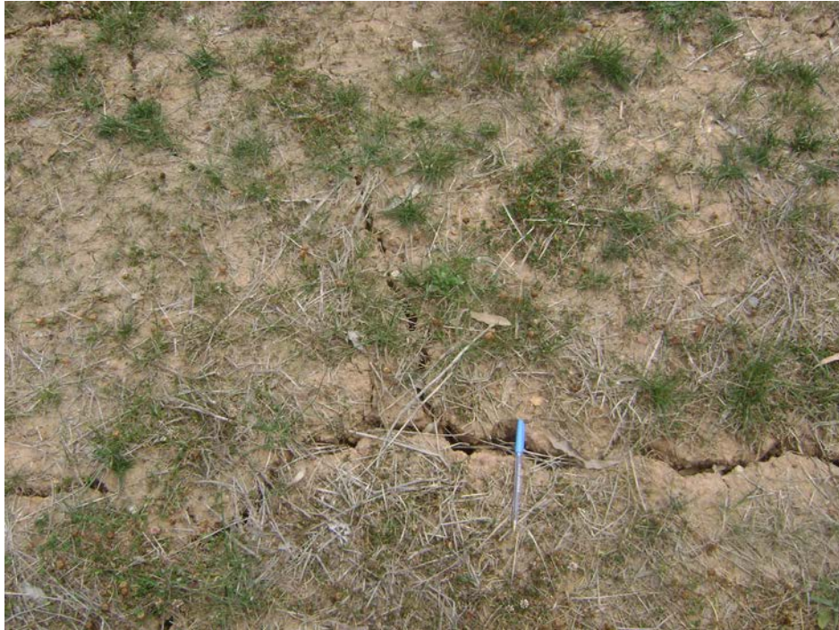
Photo 11 – Tension/shrinkage cracks up to 20mm wide and 150mm deep along crest of northern slope at proposed playing fields
