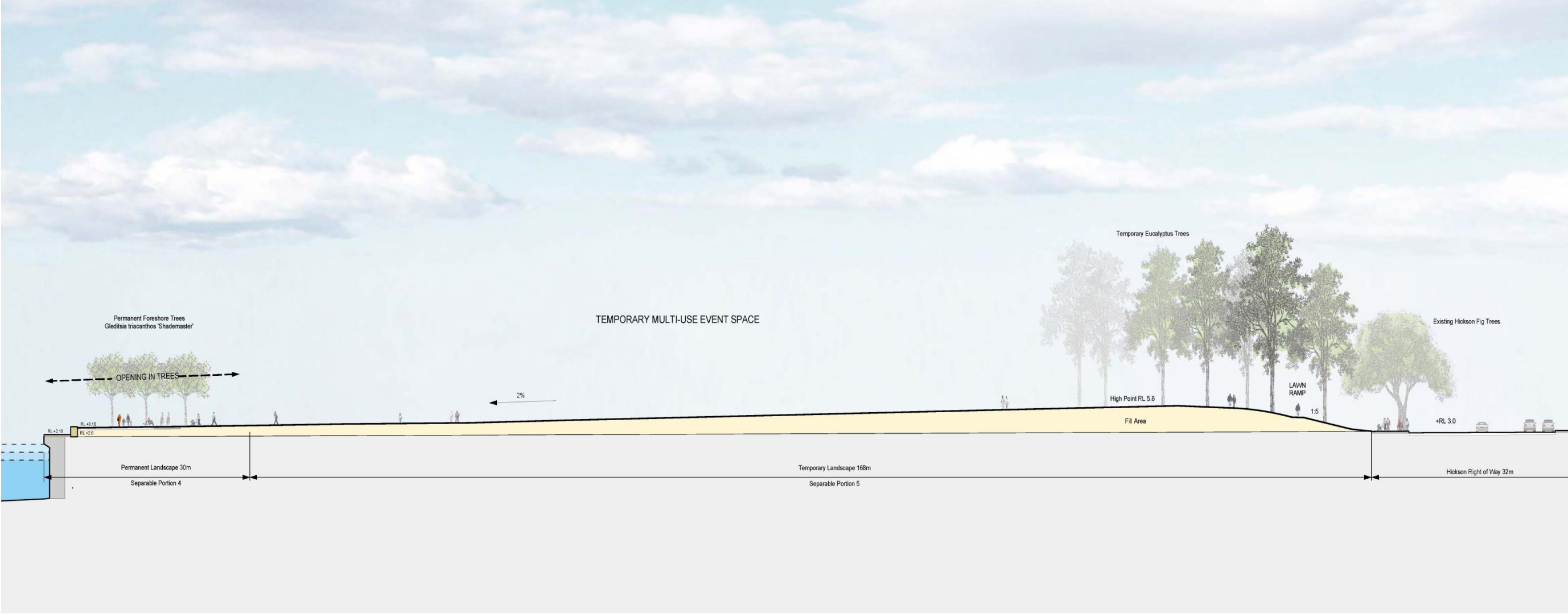
Figure 6.3 Section drawing showing the proposed profile of the Interim Public Domain. The lawn area will be filled to achieve the required slope. (Source: PWP Landscape Architecture, extract from 'Design Development Stage Two Site Sections—West East Site Section, Drawing No. TE-PWP-L-S3-8002)
