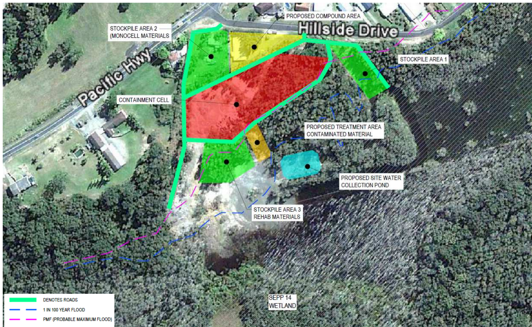
Figure 1: Proposed Works – Treatment Area, Containment Cell, Site Compound, Access Roads and Stockpiles
