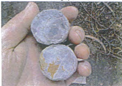
Iron staining silty clay encountered at BH2
