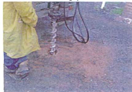
Drilling equipment in operation at BH 6
