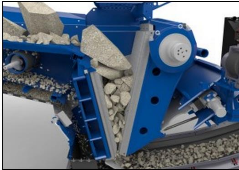
Figure 2-4 Typical Jaw Crusher Operation
