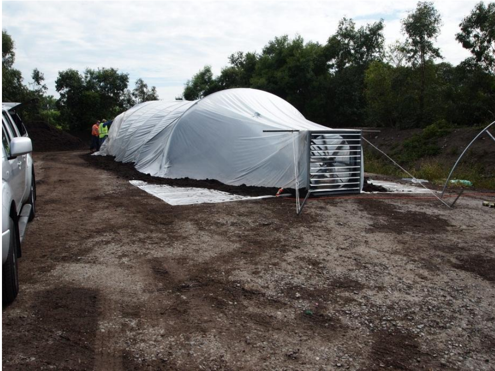
Figure 11 – Enclosed windrow for odour sampling
