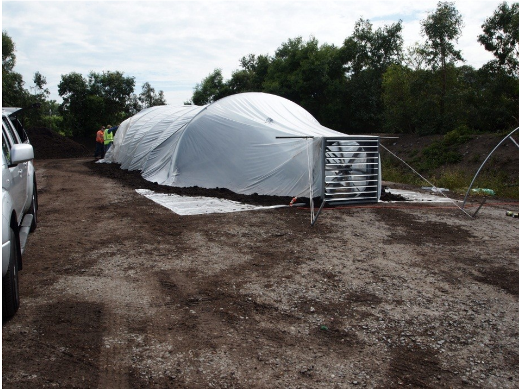
Figure 11 – Enclosed windrow for odour sampling
