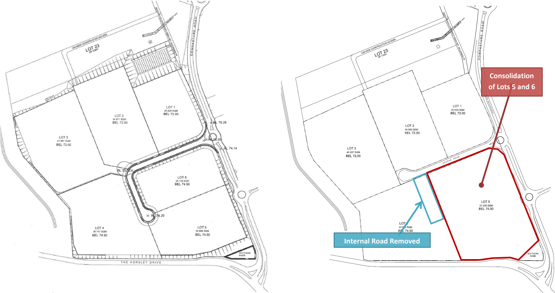
Figure 2: Comparison of Approved and Proposed Subdivision Layout (approved left, proposed right)
