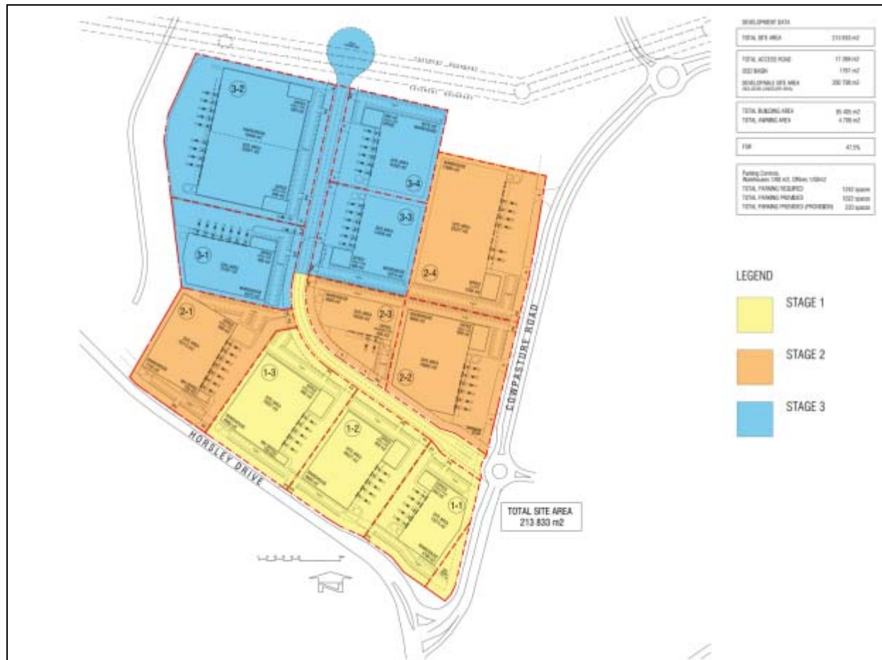
Figure 1.7: Proposed Staging of the HDBP Subdivision and Development (Source: WSP Trust 2012).
