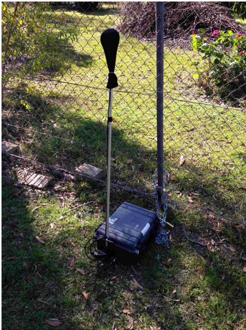
Figure 2 - Example unattended noise logger setup
