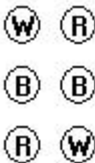
Figure 10 – Line 25/26 Phasing Arrangement – Looking Toward Eraring/Munmorah
