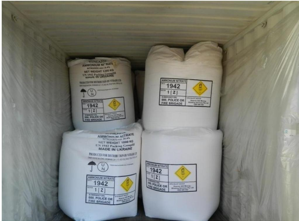
*Photograph 1.3 Stacking Arrangement inside Shipping Container within Storage Compound.*
