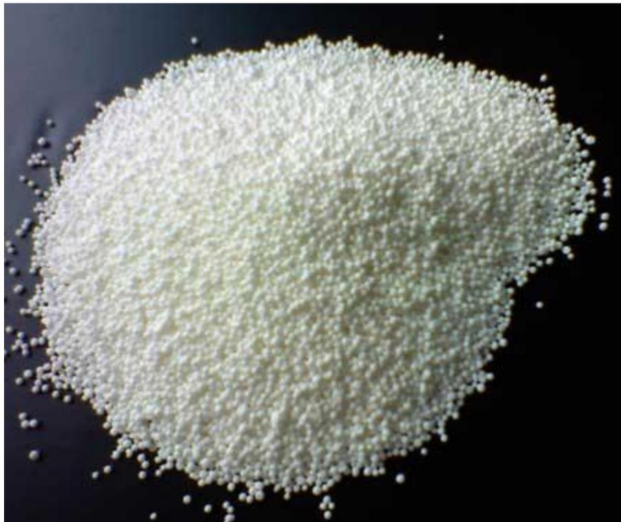
*Photograph 1.1 Example of Prilled Ammonium Nitrate*
