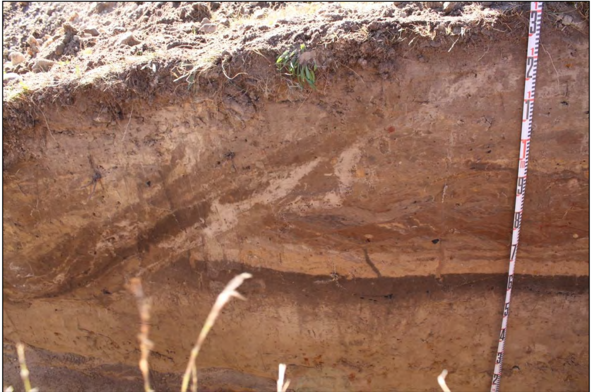
MHPAD1 Transect 8, northern profile showing layers of fill over old soil - horizon western end
