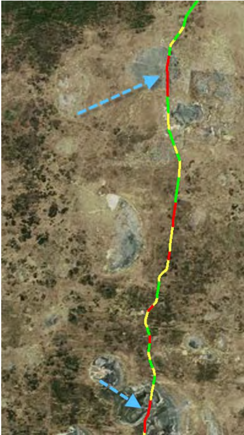
Figure 7 Poor CBR values within areas in lake crossings
