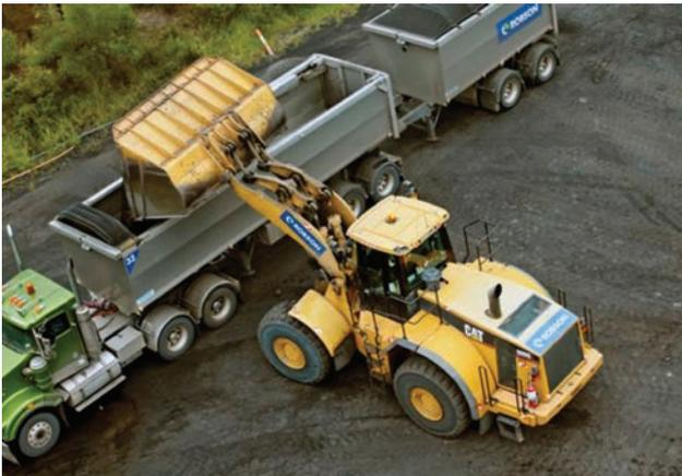
**Plate ES-2 – Loading of ROM Coal into a B-Double Truck at the Tasman Underground Mine**
