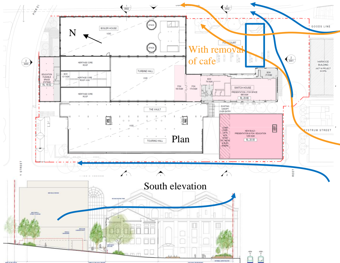
Figure 11: Sketch of flow patterns around reference design for winds from the south
