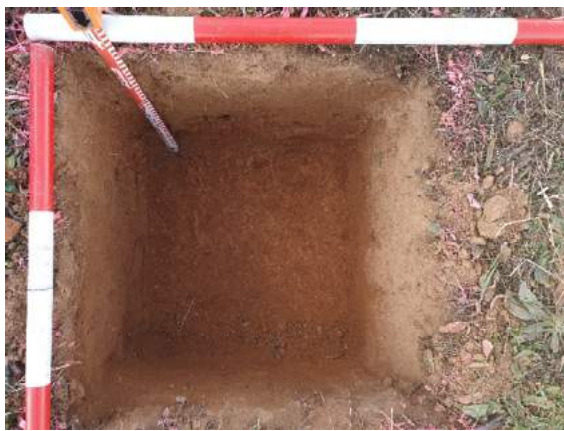
Figure 14: Test pit 6 – Plan view showing hard set decomposing siltstone at base
