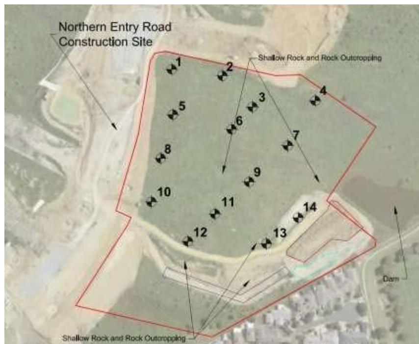
Figure 5 – Layout of Geotechnical Boreholes based on Douglas Partners Report
