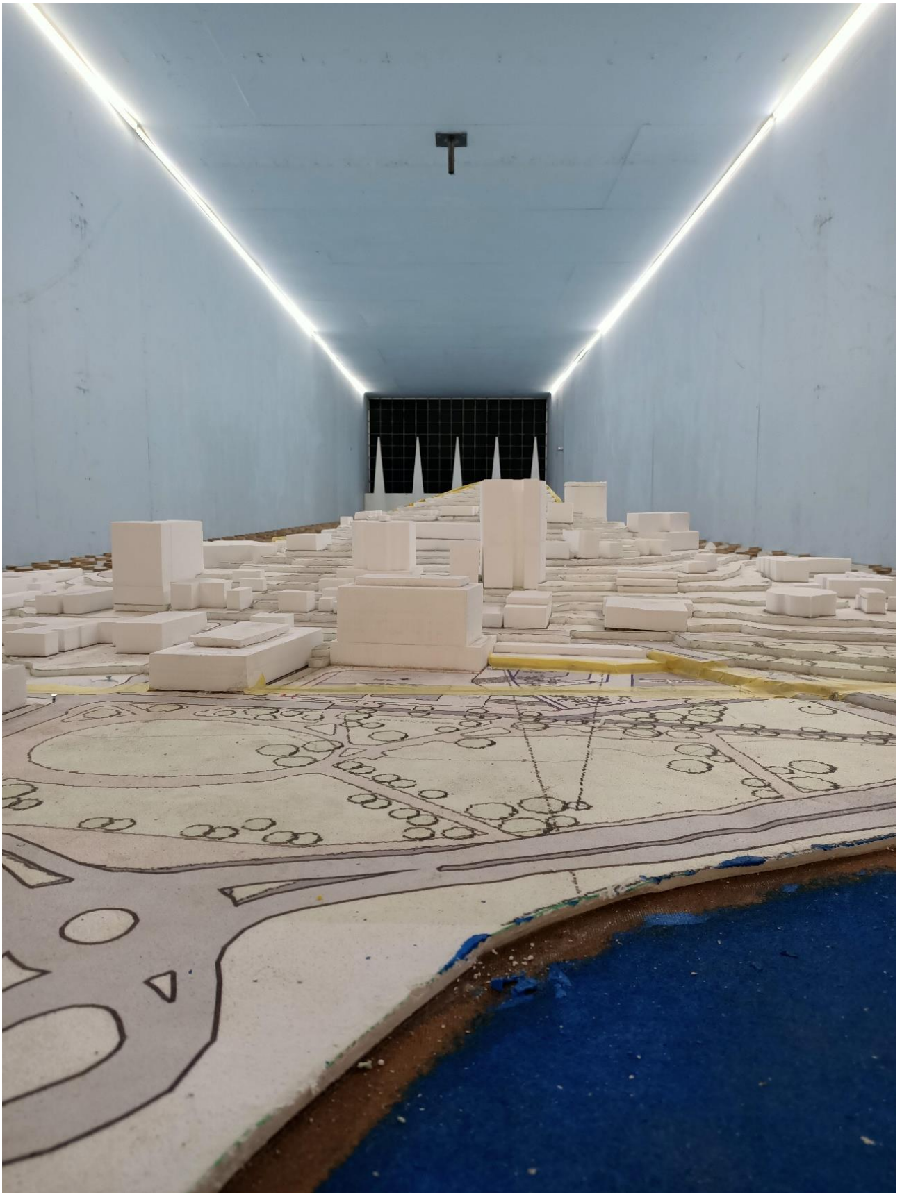
Figure 1k: Photograph of the Wind Tunnel Model (Existing Scenario - view from the west)
