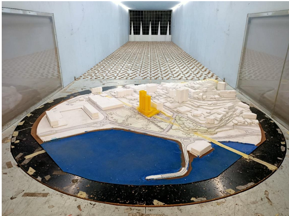
Figure 1d: Photograph of the Wind Tunnel Model (Proposed Scenario - view from the south-west)
