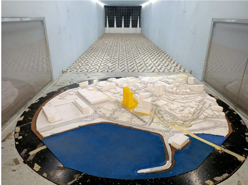
Figure 1i: Photograph of the Wind Tunnel Model (Future Scenario - view from the south-west)
