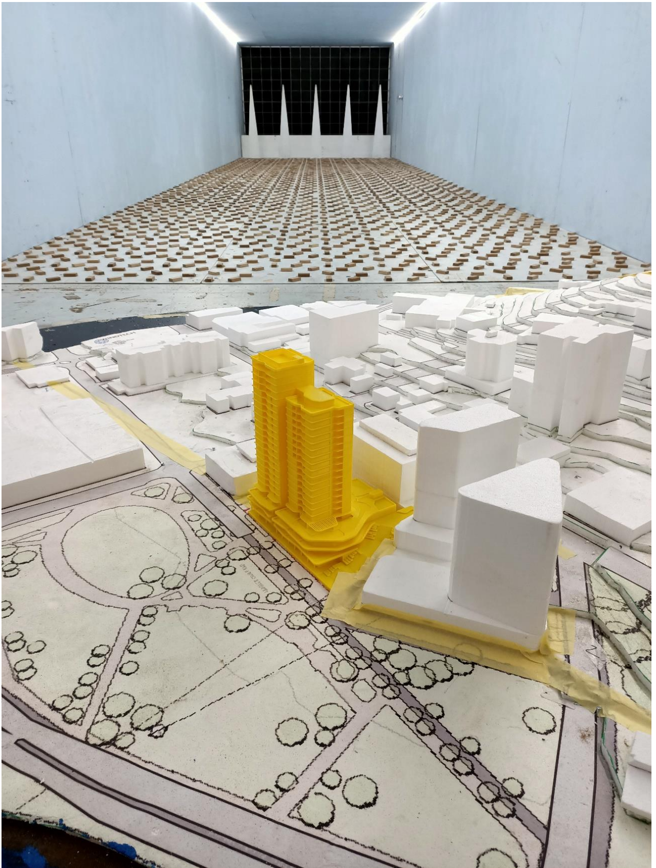
Figure 1f: Photograph of the Wind Tunnel Model (Future Scenario - view from the south-west)
