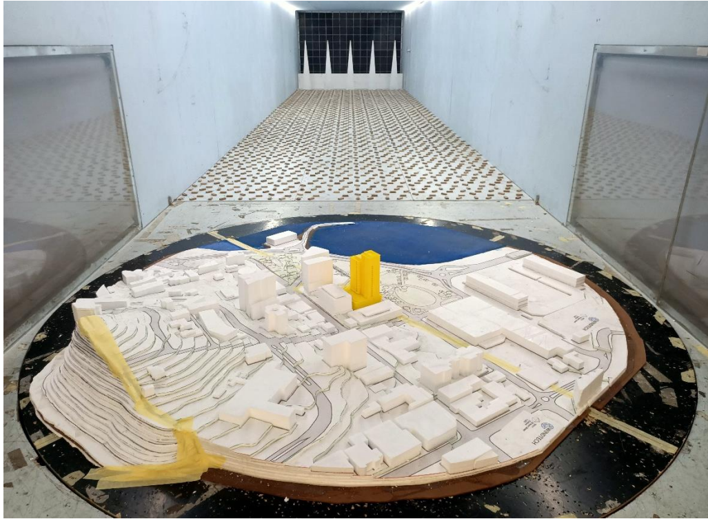
Figure 1g: Photograph of the Wind Tunnel Model (Future Scenario - view from the north-east)
