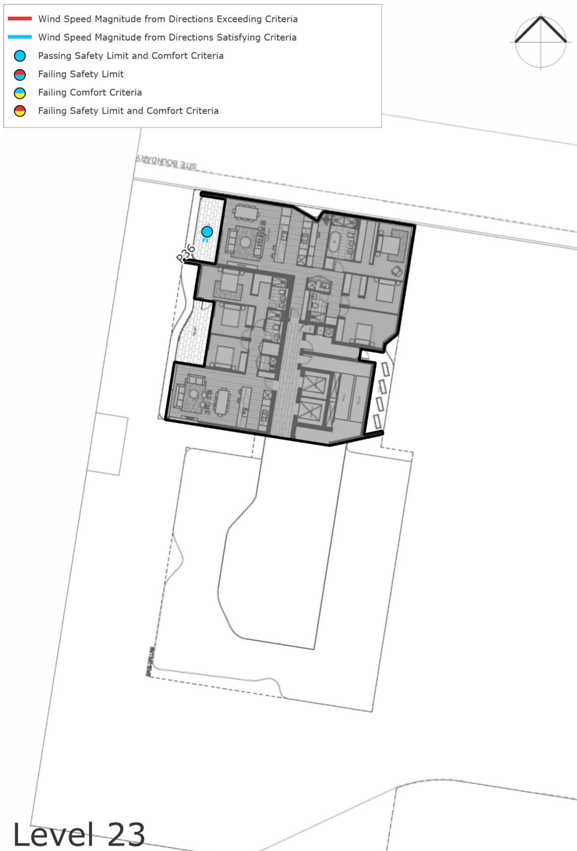
Figure 60: Wind Tunnel Results – Future Scenario – Level 23 (results shown without treatments applied)
