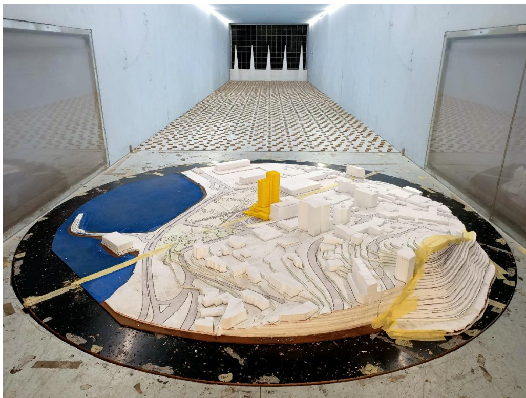
Figure 1c: Photograph of the Wind Tunnel Model (Proposed Scenario - view from the south-east)
