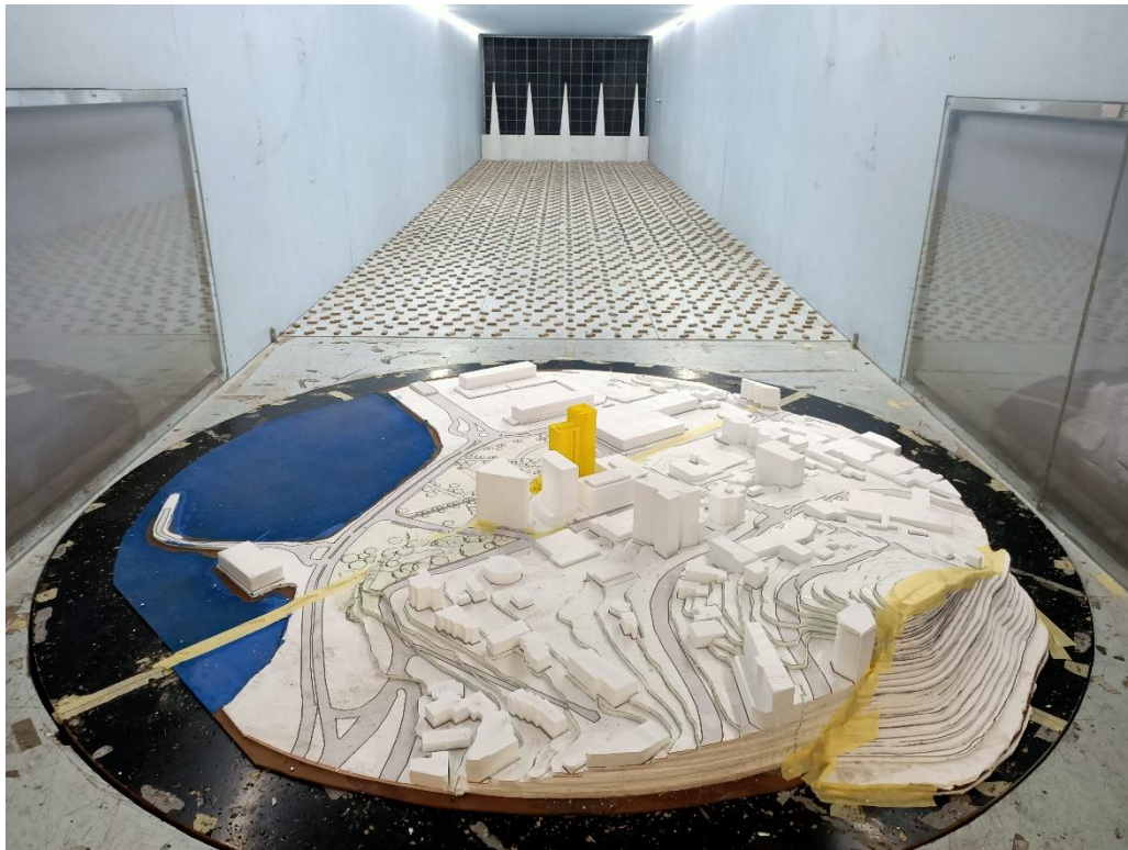
Figure 1h: Photograph of the Wind Tunnel Model (Future Scenario - view from the south-east)
