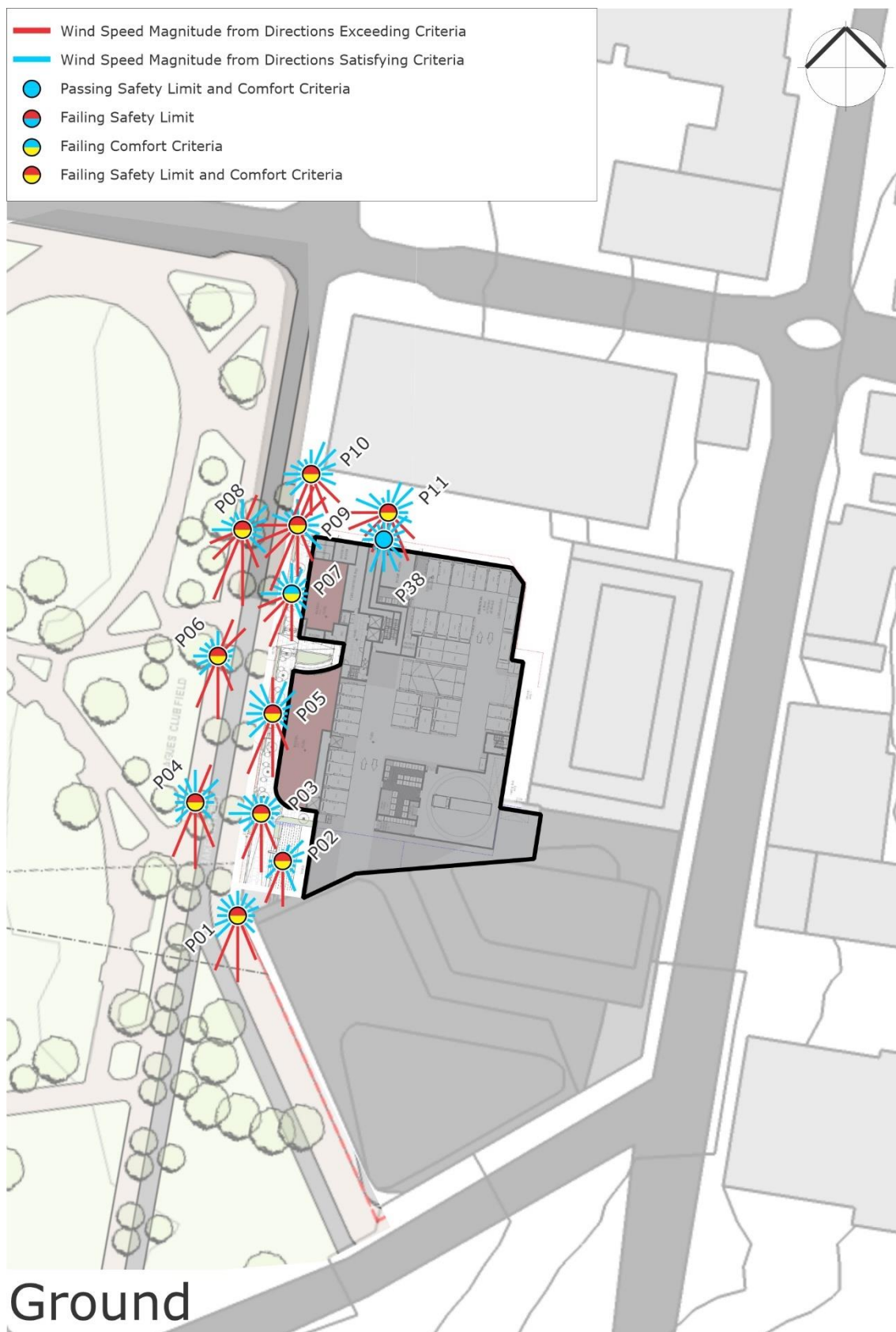
Figure 6i: Wind Tunnel Results – Future Scenario – Ground Floor (results shown without treatments applied)
