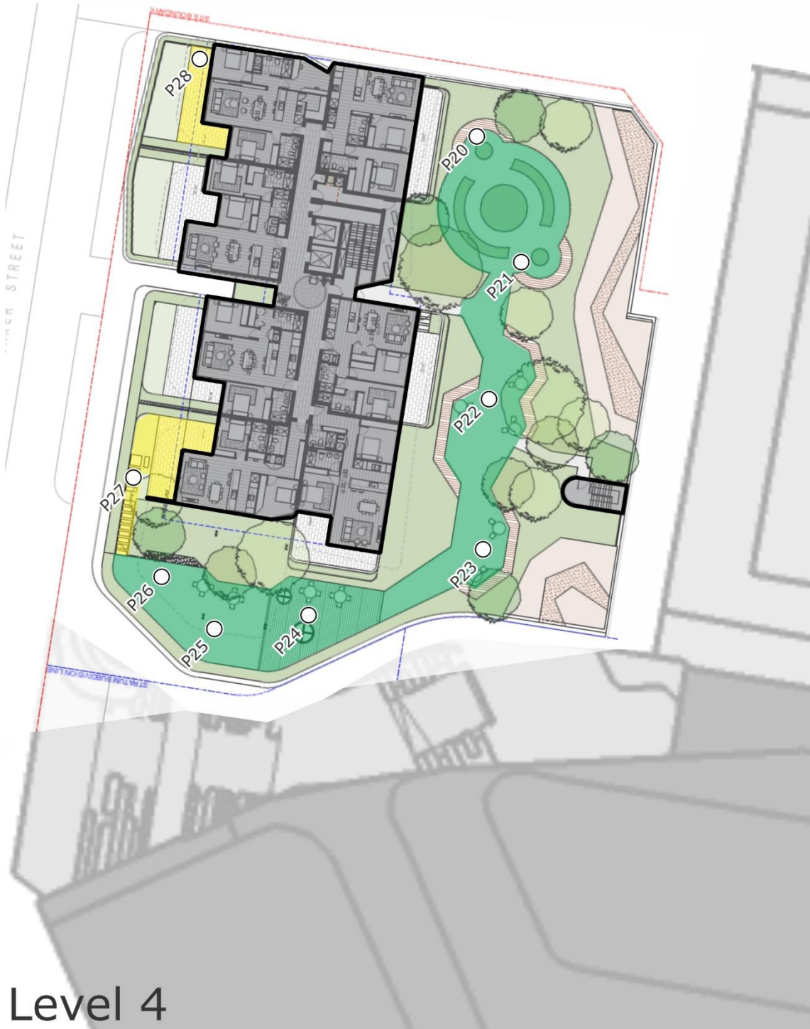
Figure 5d: Study Point Locations and Target Wind Speed Criteria – Level 4 Plan
