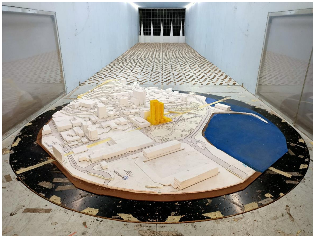
Figure 1e: Photograph of the Wind Tunnel Model (Proposed Scenario - view from the north-west)
