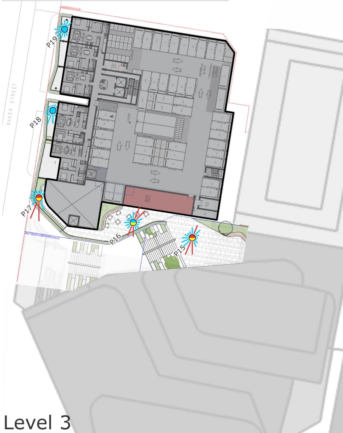
Figure 6k: Wind Tunnel Results – Future Scenario – Level 3 (results shown without treatments applied)
