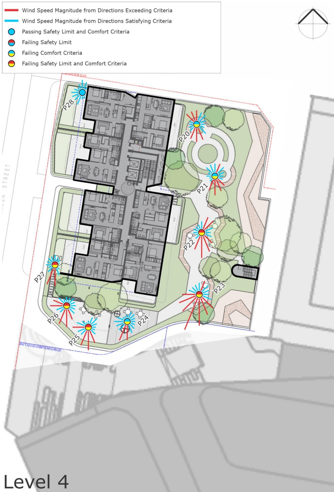
Figure 6l: Wind Tunnel Results – Future Scenario – Level 4 (results shown without treatments applied)
