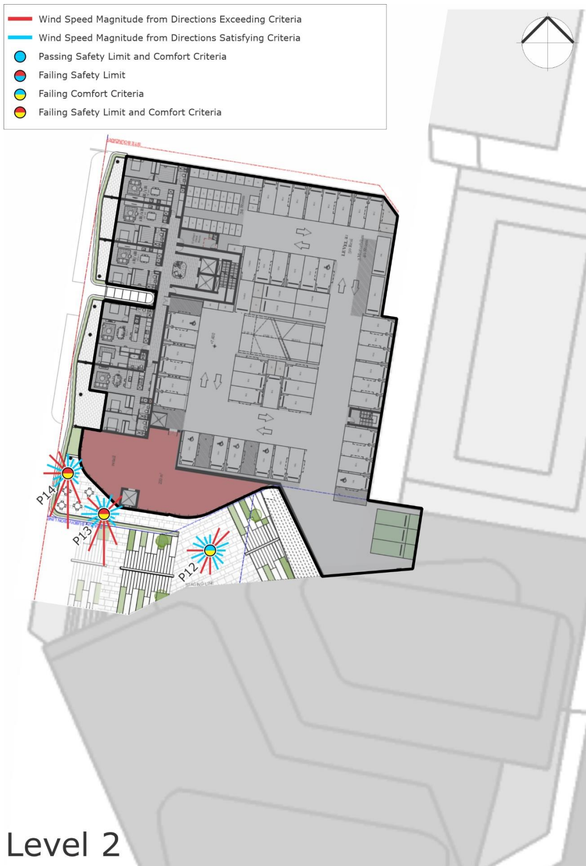
Figure 6j: Wind Tunnel Results – Future Scenario – Level 2 (results shown without treatments applied)
