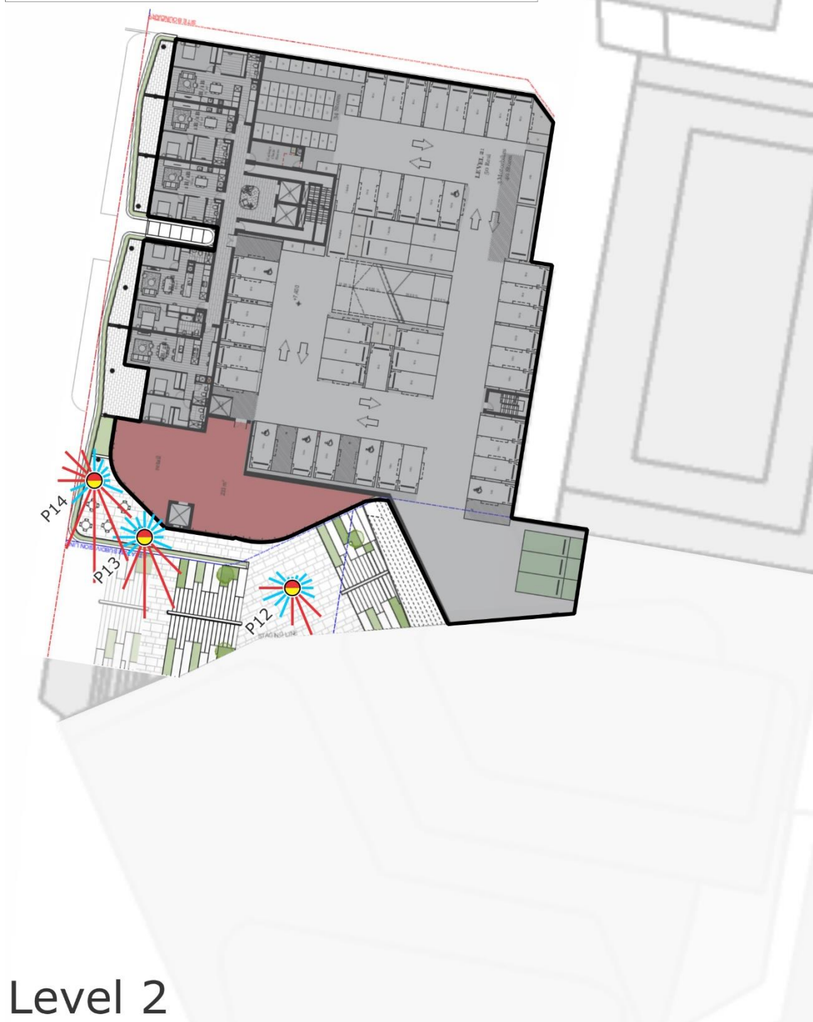
Figure 6b: Wind Tunnel Results – Proposed Scenario – Level 2 (results shown without treatments applied)
