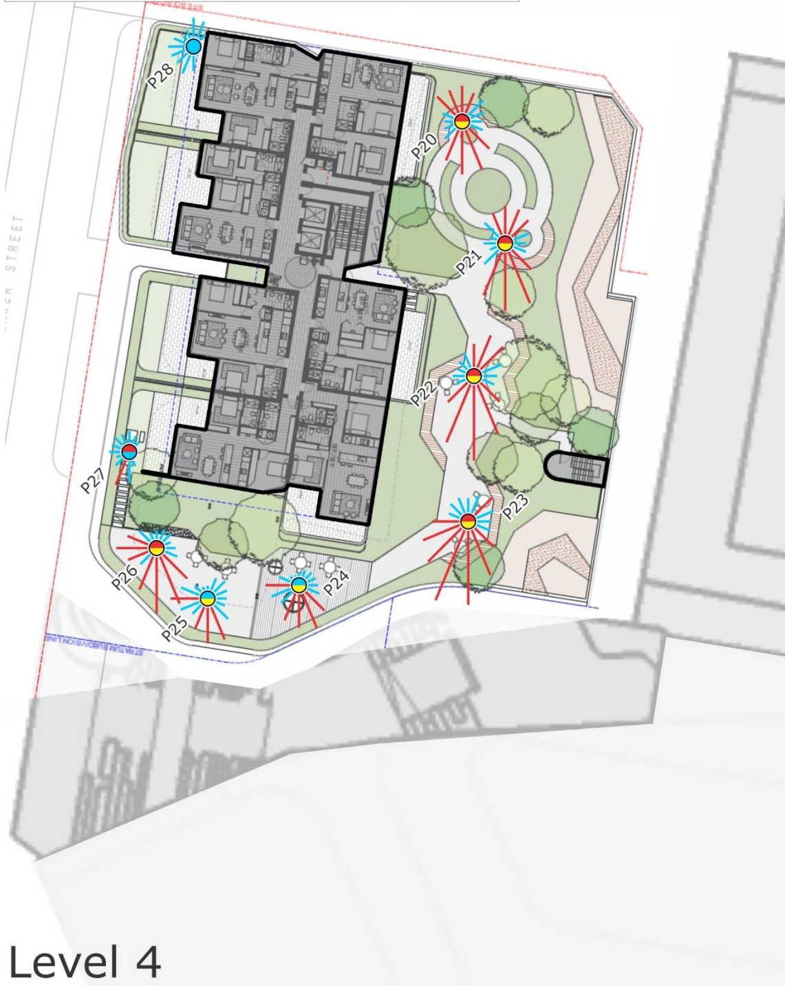
Figure 6d: Wind Tunnel Results – Proposed Scenario – Level 4 (results shown without treatments applied)
