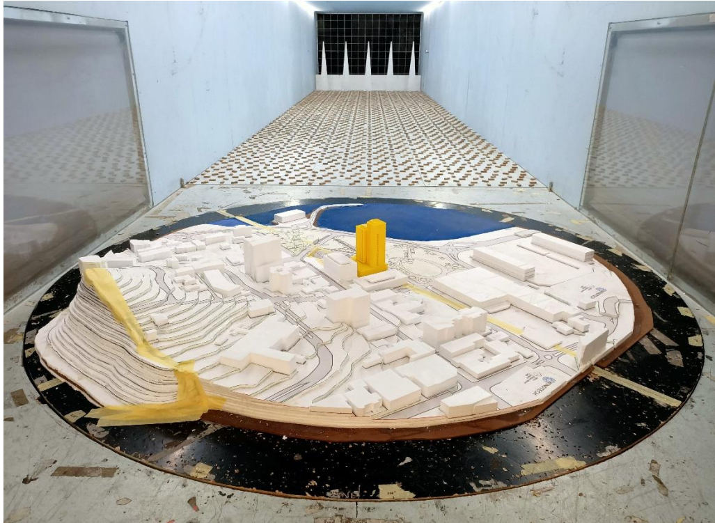
Figure 1b: Photograph of the Wind Tunnel Model (Proposed Scenario - view from the north-east)
