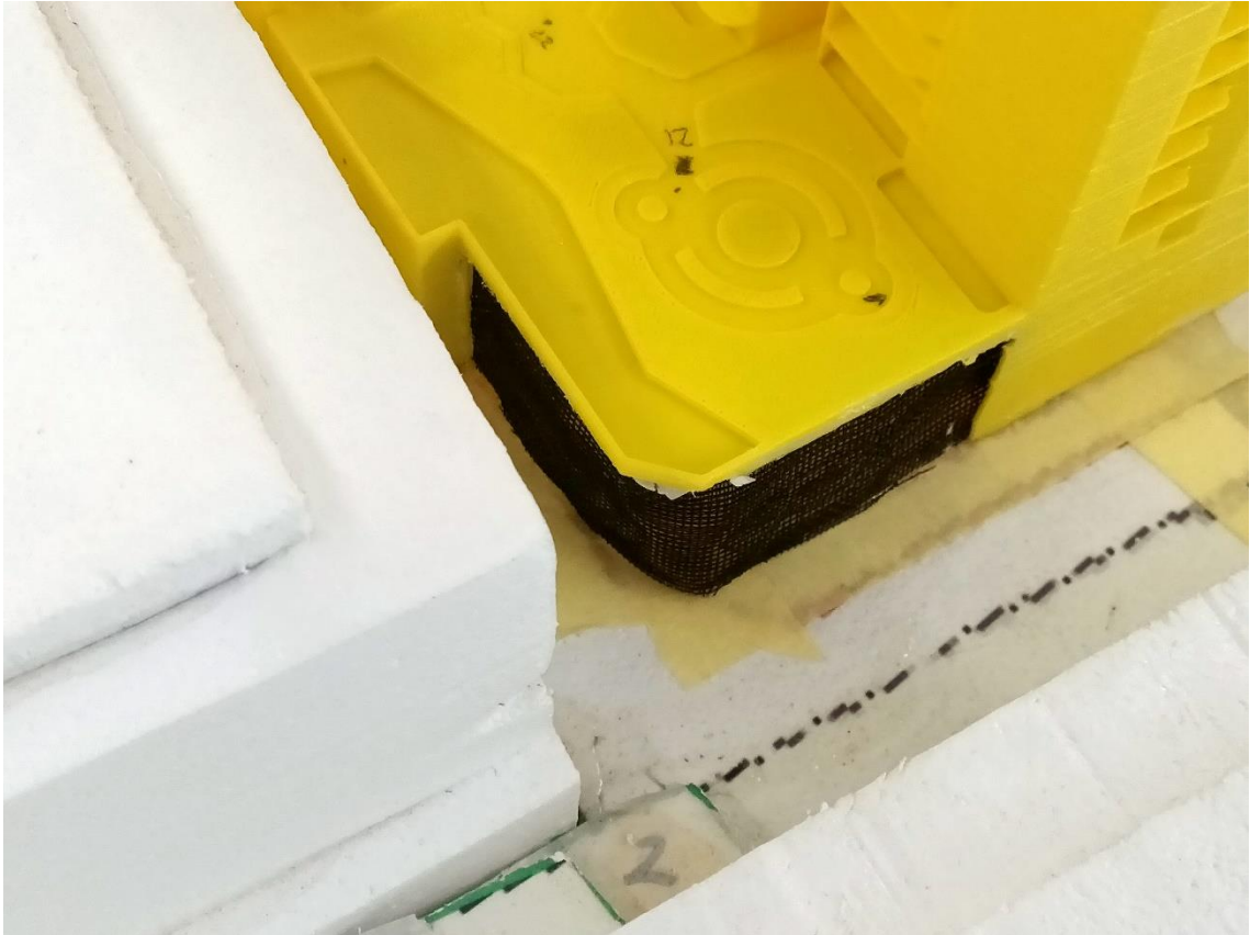
Figure C.2: Photograph of the Wind Tunnel Model with porous carpark facade
