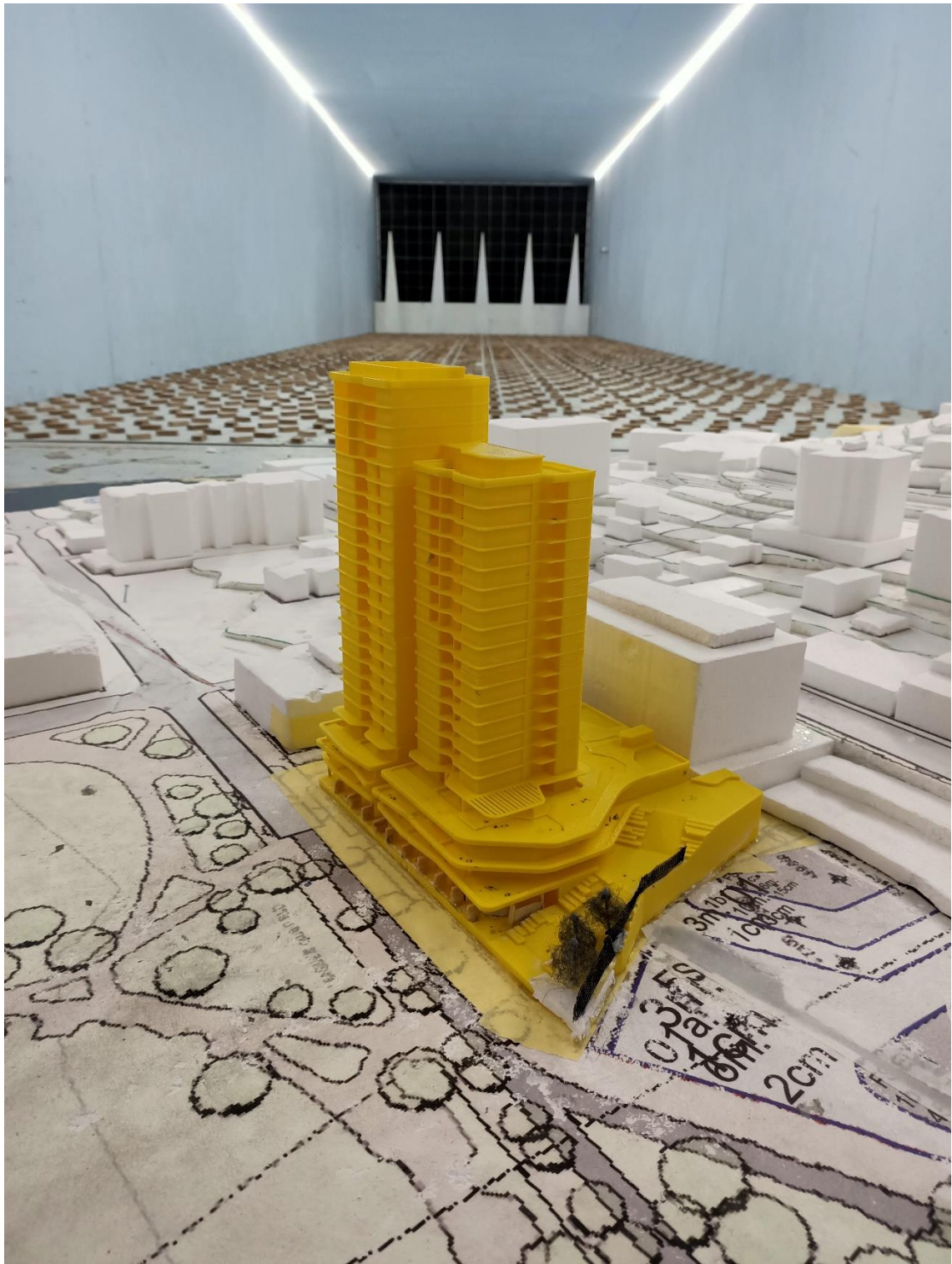
Figure C.3: Photograph of the Wind Tunnel Model with Option 2 café seating treatments, 2m high 30% porous screen running along southern edge from ground to Level 2, 3-4m high trees in planter area
