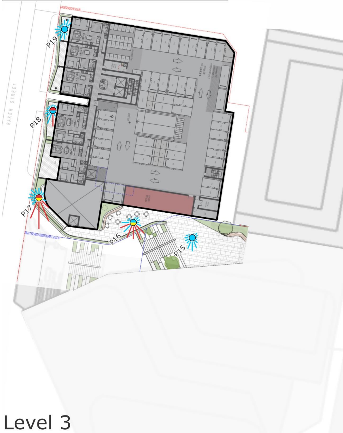
Figure 6c: Wind Tunnel Results – Proposed Scenario – Level 3 (results shown without treatments applied)
