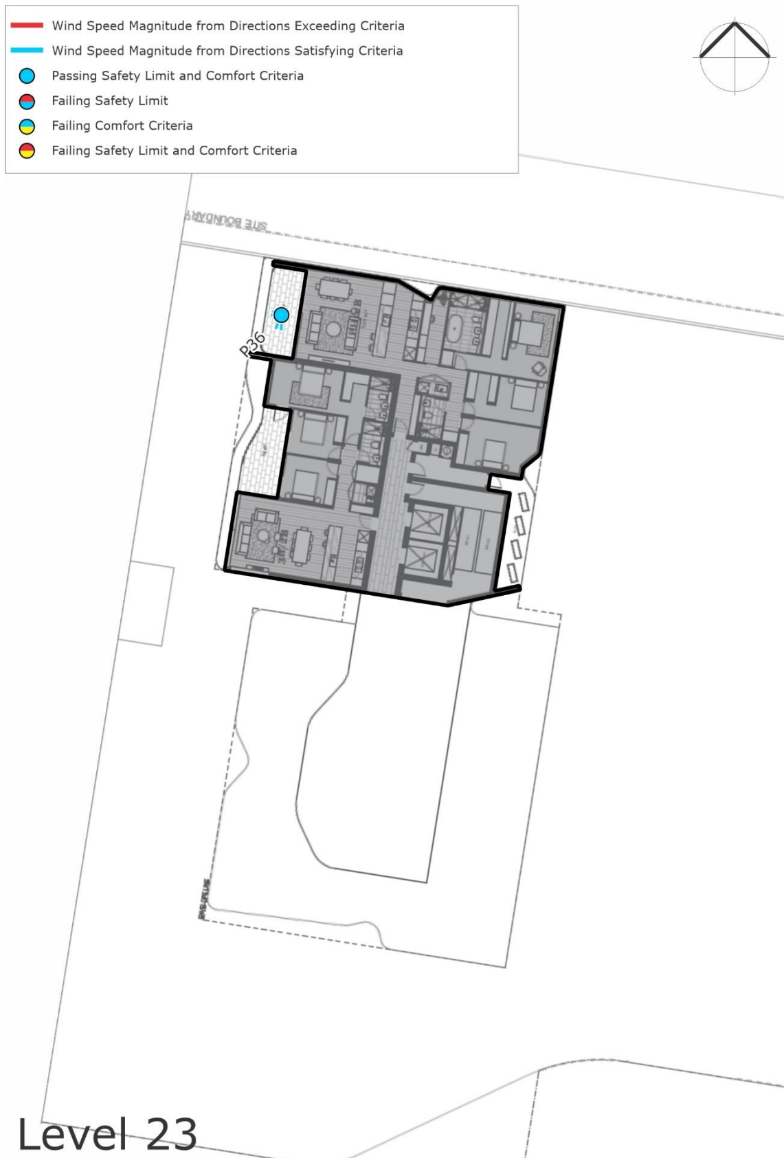
Figure 6g: Wind Tunnel Results – Proposed Scenario – Level 23 (results shown without treatments applied)
