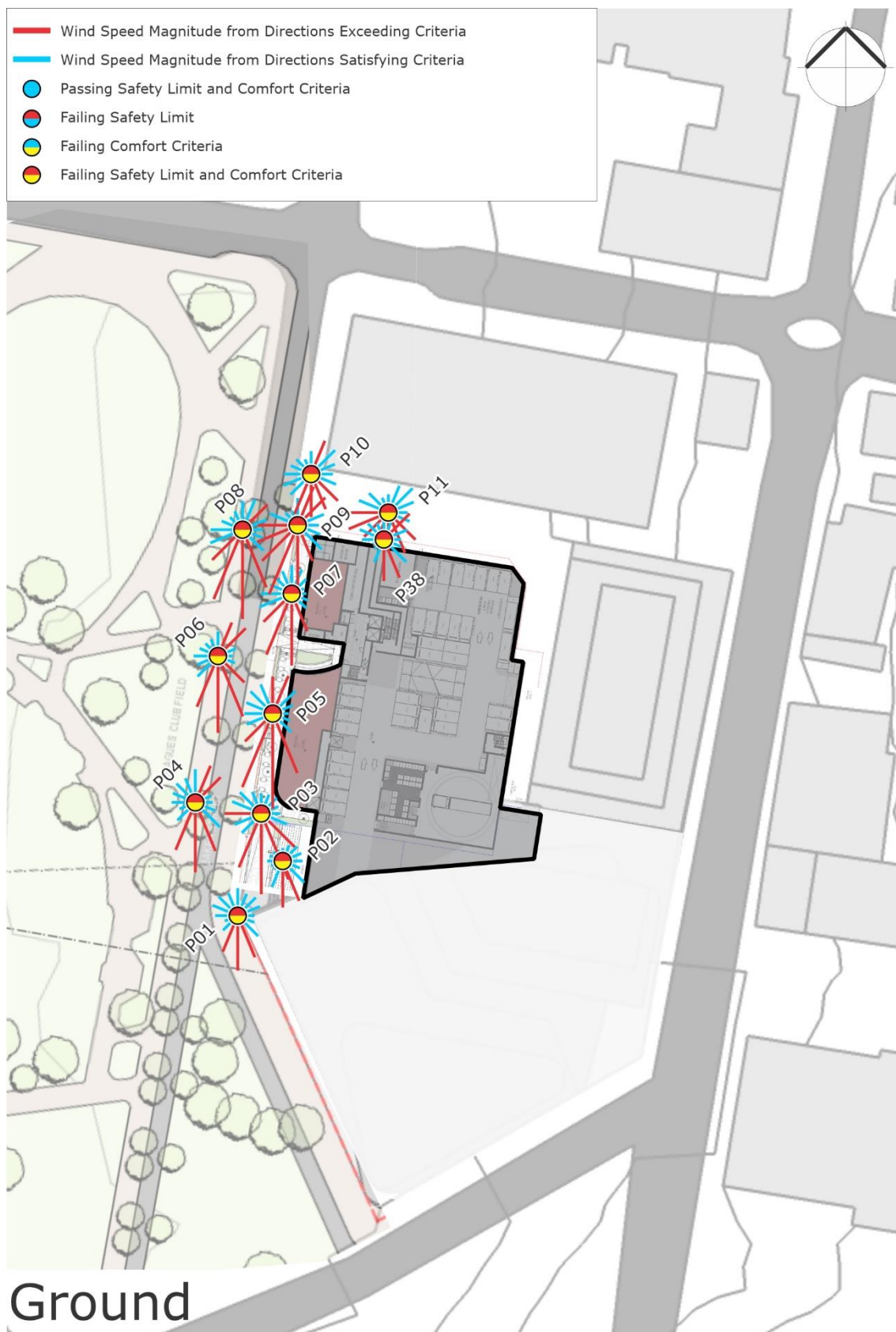
Figure 6a: Wind Tunnel Results – Proposed Scenario - Ground Floor (results shown without treatments applied)
