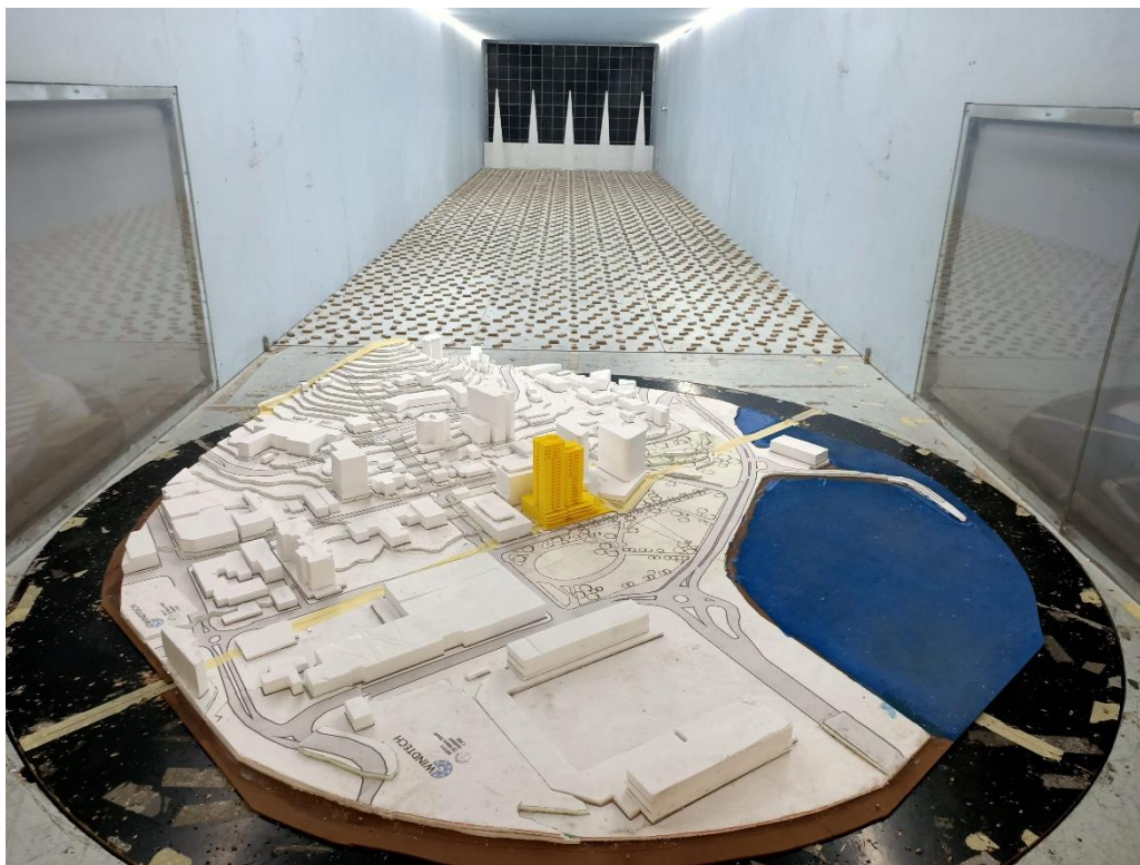
Figure 1j: Photograph of the Wind Tunnel Model (Future Scenario - view from the north-west)
