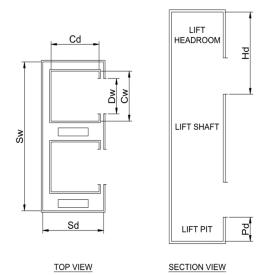
LIFT CAR DIMENSIONS INTERNAL SHAFT DIMENSIONS Width Car Door Car Width Car Depth Internal Depth (Sd) Headroom Pit Depth Group Door Width Height (Cw) (Cd) Car (Sw) (Hd) (Pd) (Dw) Height 4,850mm Duplex 1,000mm/ including 2,300mm 1,450mm 2,000mm 2,500mm 2,450mm 5,200mm 2,400mm (2) 1.100mm trimmer beam
