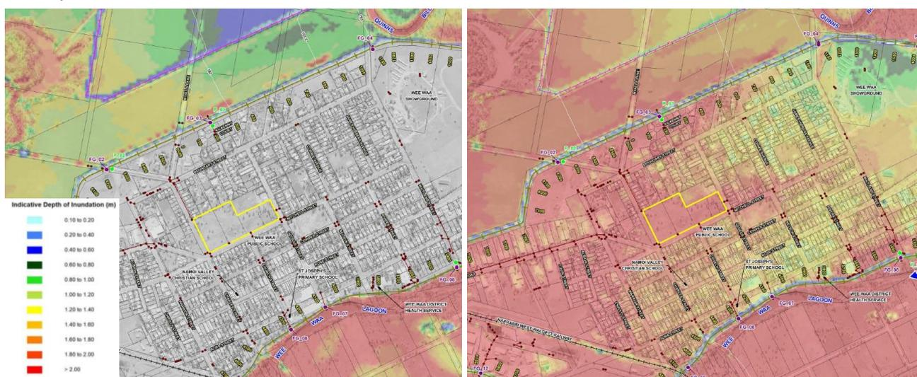
**Figure 13 Existing Site Flood Inundation Levels for Riverine Flooding: 1% AEP (left), Extreme (right)**
