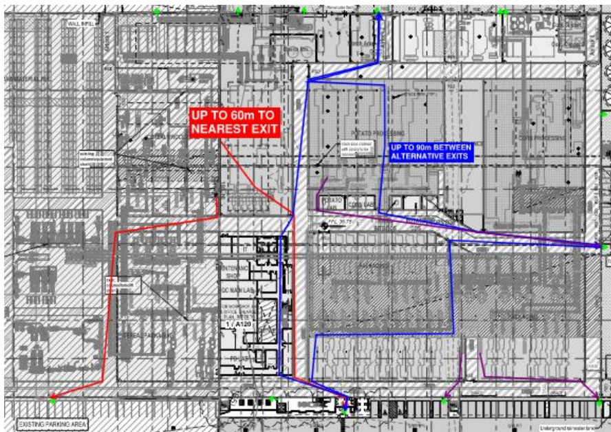
Figure 4.5 – Extended Travel Distances in Warehouse and Manufacturing – Ground Floor
