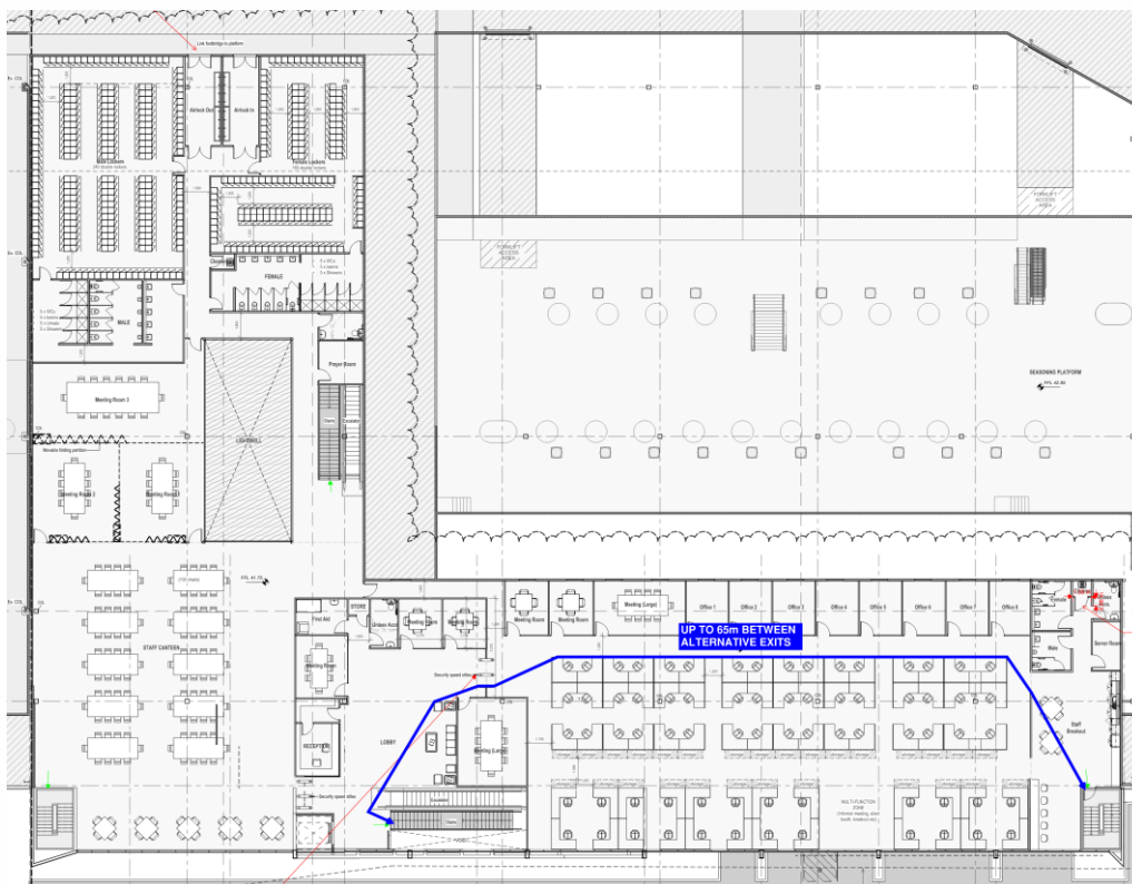
Figure 4.6 – Extended Travel Distances in New Office – Ground Floor
