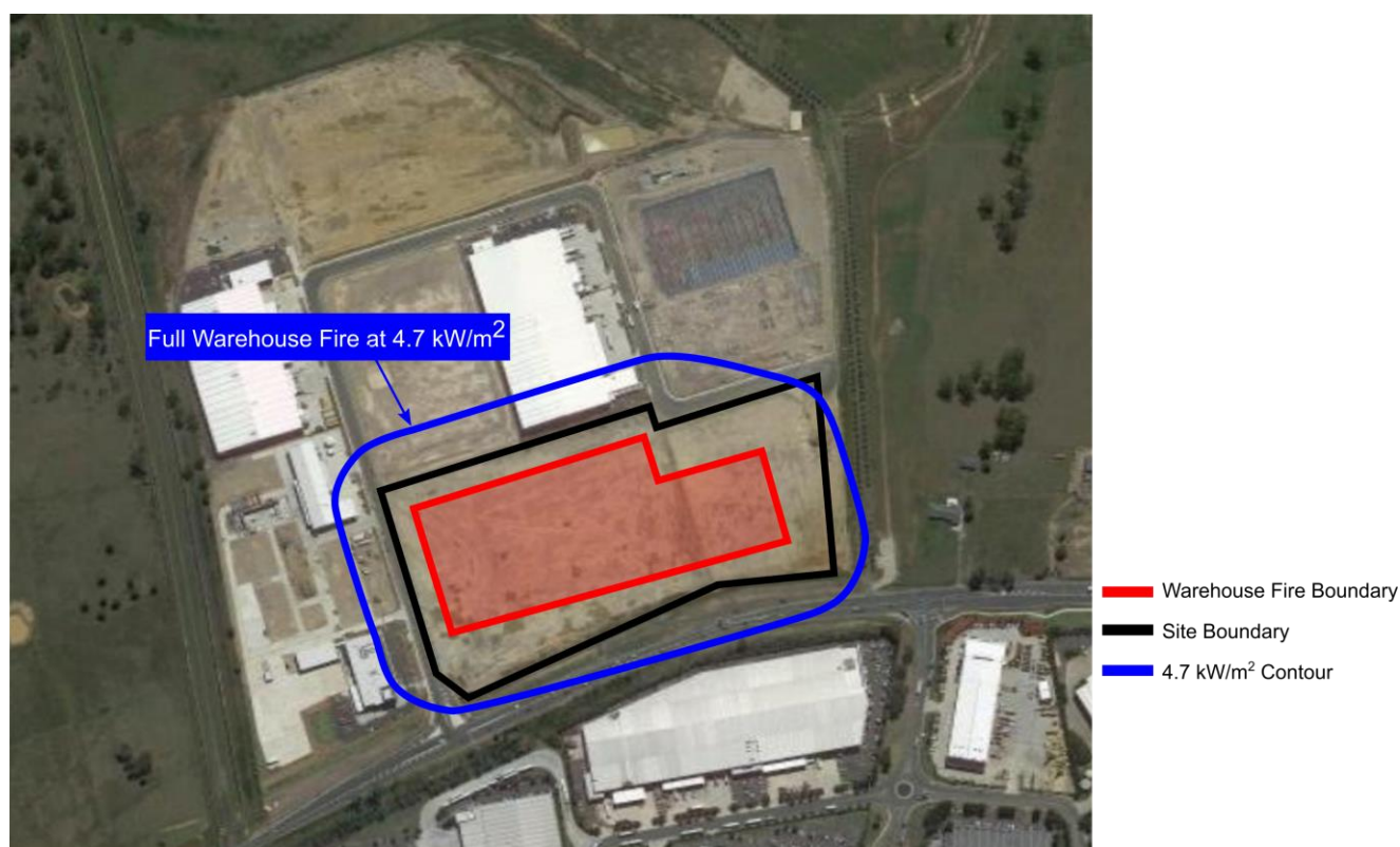
Figure 5-2: Full Warehouse Fire Radiant Heat Contours
