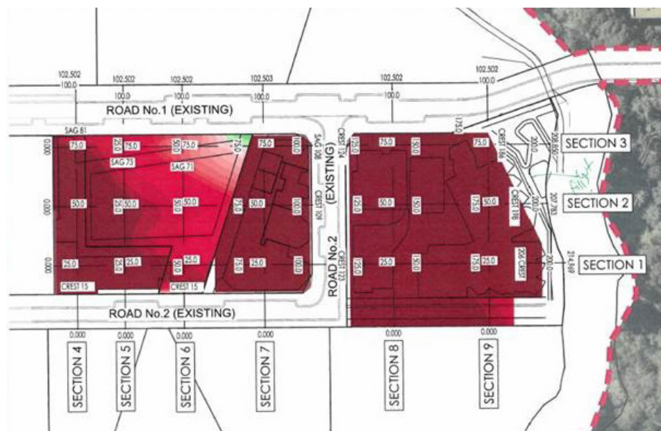
Figure 8 Extract of cut and fill plan
