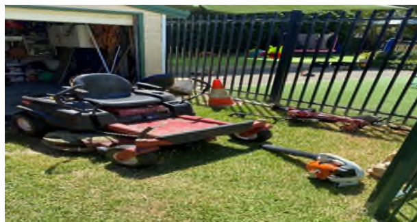
Photograph 12: Lawn maintenance equipment used by groundskeepers. ULP powered lawn mower, blower and edger.
