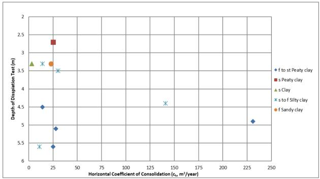
Figure 1: Graph of ch vs. Depth for various material types
