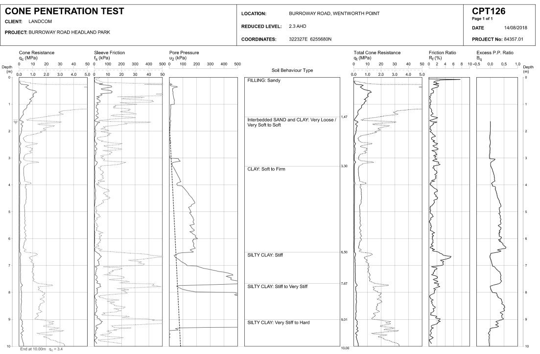
**REMARKS:** HAND AUGER TO 0.3 m. TEST DISCONTINUED AT TARGET DEPTH. GROUNDWATER OBSERVED AT 1.65 m AFTER WITHDRAWAL OF RODS.
