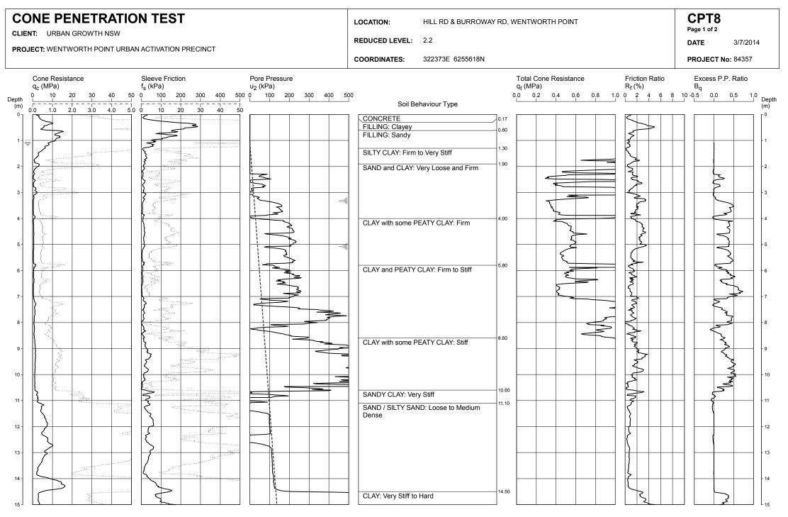
REMARKS: HOLE COLLAPSE AT 1.1 m DEPTH AFTER WITHDRAWAL OF RODS.
