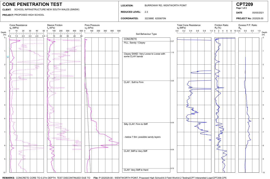
BENDING ON INFERRED WEATHERED ROCK. GROUNDWATER OBSERVED AT 1.45m AFTER WITHDRAWAL OF RODS.
