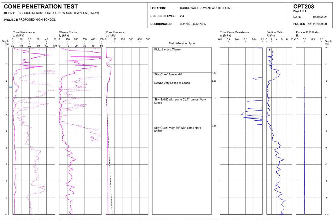
REMARKS: TEST DISCONTINUED DUE TO REFUSAL ON INFERRED WEATHERED File: P:\202029.00 - WENTWORTH POINT, Proposed High School\4.0 Field Work\4.2 Testing\CPT Interpreted Logs\CPT203.CP5 Cone ID: 200309T Type: I-CFXYP20-10 ROCK.
