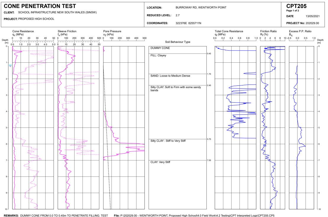
REMARKS: DUMMY CONE FROM 0.0 TO 0.45m TO PENETRATE FILLING. TEST File: P:\202029.00 DISCONTINUED DUE TO REFUSAL ON INFERRED WEATHERED ROCK.Cone ID: 120522T GROUNDWATER OBSERVED AT 1.2m AFTER WITHDRAWAL OF RODS.
