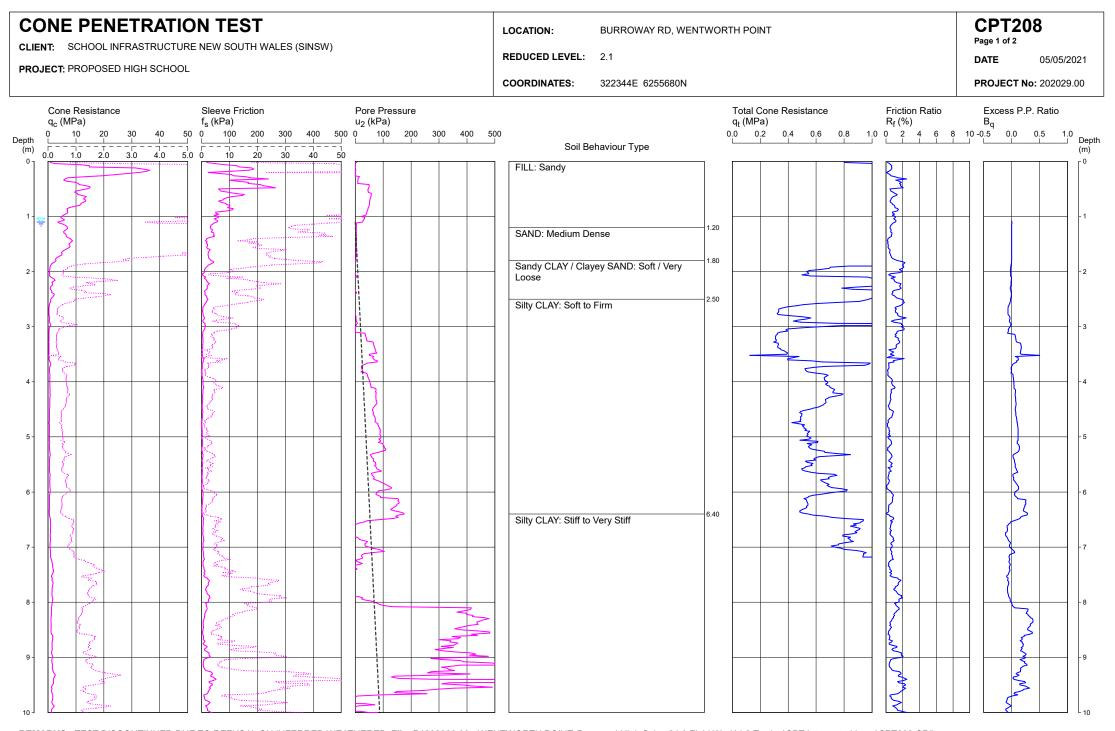
REMARKS: TEST DISCONTINUED DUE TO REFUSAL ON INFERRED WEATHERED File: P:\202029.00 - WENTWORTH POINT, Proposed High School\4.0 Field Work\4.2 Testing\CPT Interpreted Logs\CPT208.CP5 ROCK.GROUNDWATER OBSERVED AT 1.1m AFTER WITHDRAWAL OF ROD&ID: 120522T Type: I-CFXYP20-10
