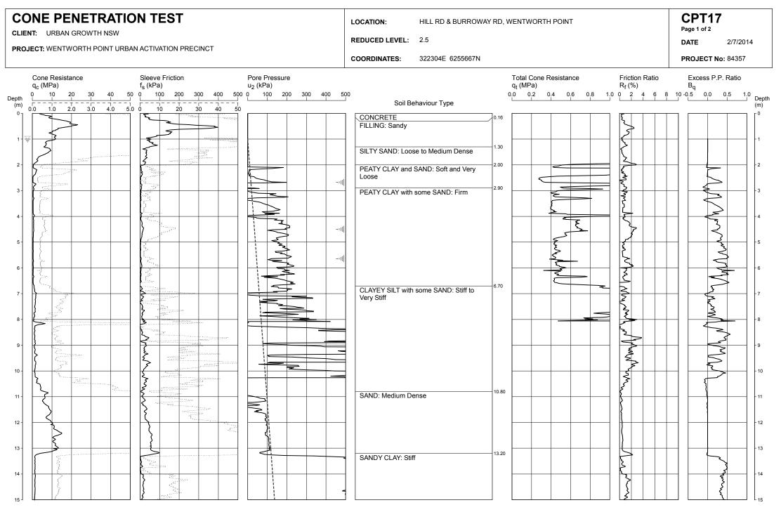
**REMARKS:** HOLE COLLAPSE AT 0.5 m DEPTH AFTER WITHDRAWAL OF RODS.
