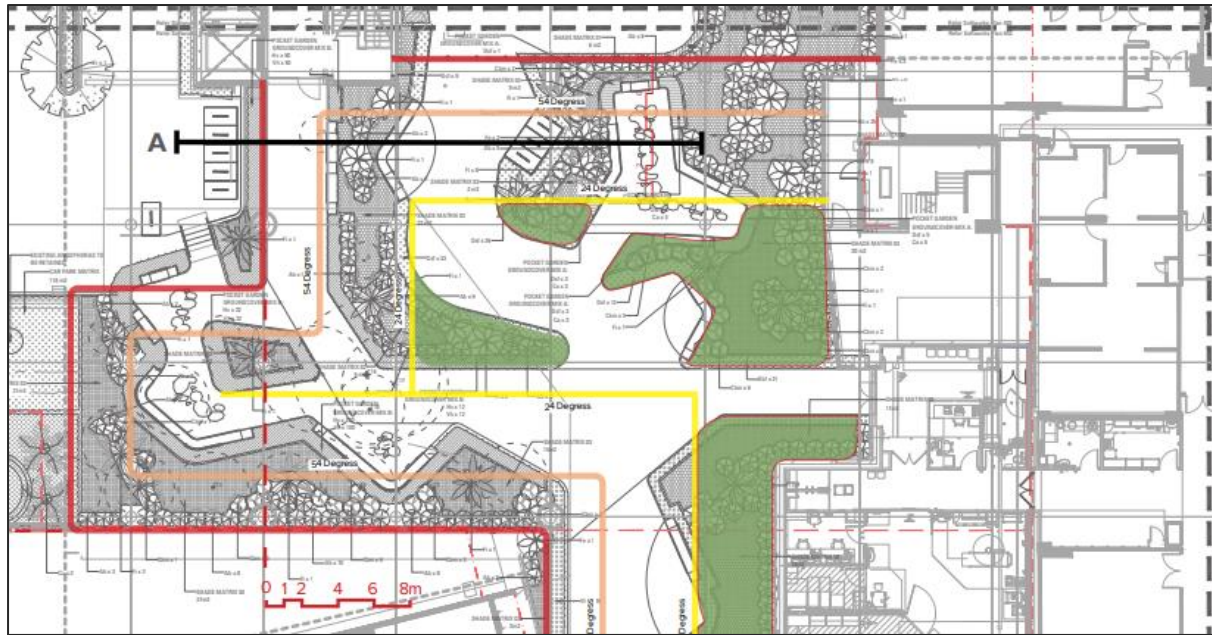
Figure 25 | Plan of undercroft area, demonstrating the building overhang (red), summer sun angle (peach) and winter sun angle (yellow) (Source: Applicant's RtS).
