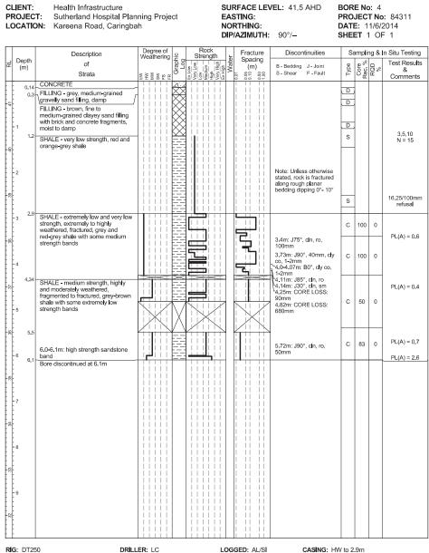
TYPE OF BORING: Diatube to 0.14m; Solid flight auger to 2.9m; NMLC-Coring to 6.1m WATER OBSERVATIONS: No free groundwater observed whilst augering
