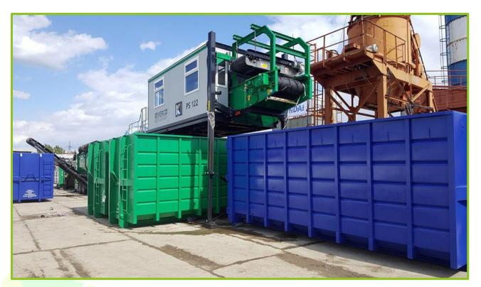
FIGURE 12 TYPICAL ELEVATED MANUAL PICKING LINE FOR SORTING OF WASTE WOOD/TIMBER
