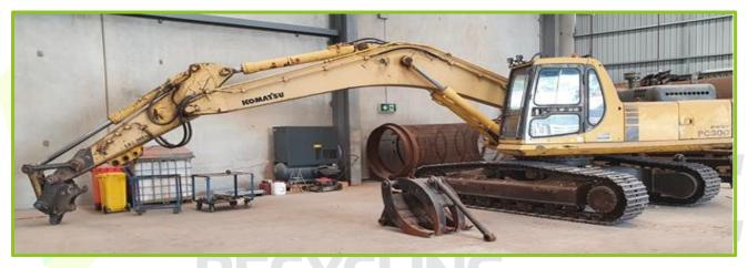
FIGURE 10 TYPICAL EXCAVATOR USED FOR MOVING AND MINIMISING WASTE WOOD AND PLASTERBOARD
