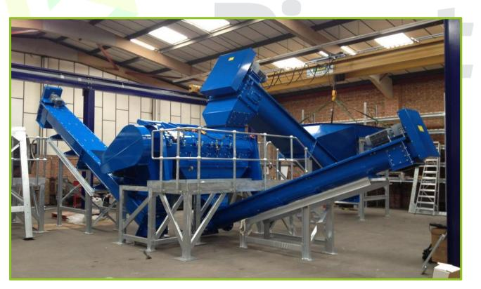
FIGURE 13 TYPICAL TURBO SEPARATOR USED FOR PROCESSING WASTE PLASTERBOARD
