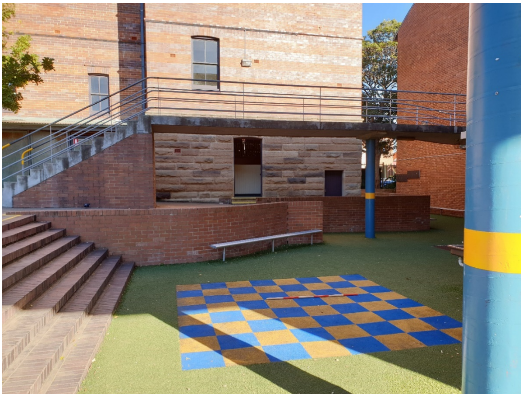
Figure 5.5 View to the south with buildings A (centre) and building E (to the right), the level of earthworks can be seen clearly as the ground level building A was constructed on is approximately 0.5m above the level building E was constructed on.
