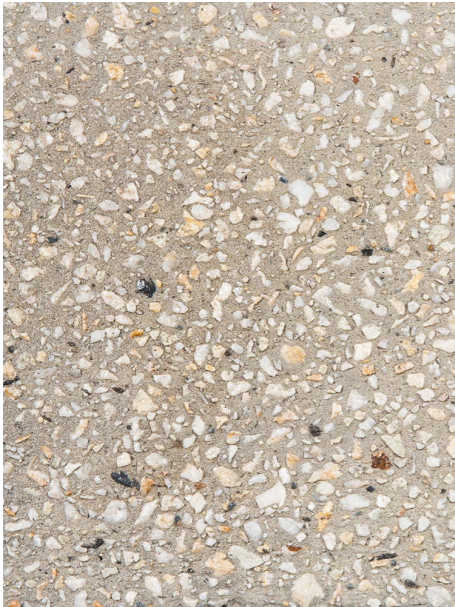
CONCRETE PAVEMENT LIGHTLY EXPOSED AGGREGATE CONCRETE. FINISH TO COMPLY WITH P4 SLIP RATING FOR GENERAL PAVEMENT, P5 FOR STEPS AND RAMPS.
