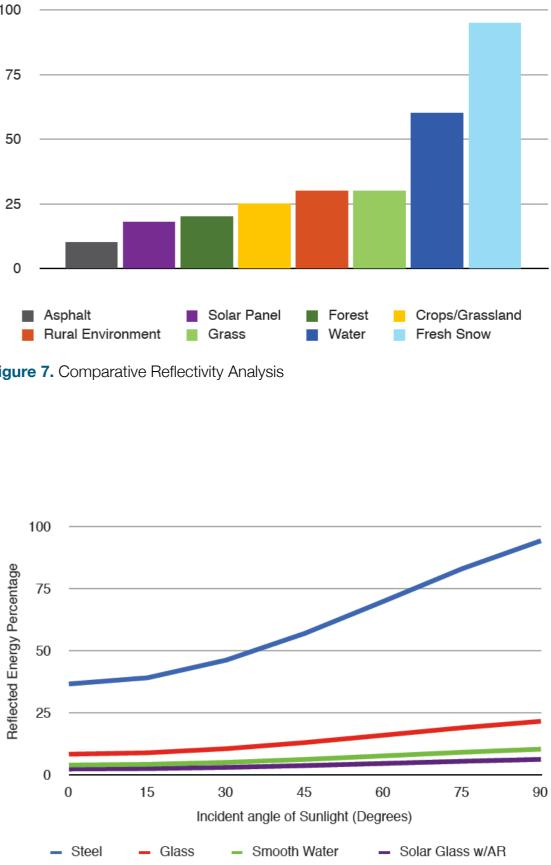
Figure 8. Analysis of Typical Material Reflectivity
