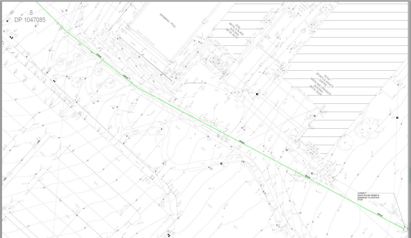
Figure 25-Image that show the proposed House sewer drainage alignment and connection to the Existing Sydney Water DN300mm sewer in the vicinity of Mars Creek
