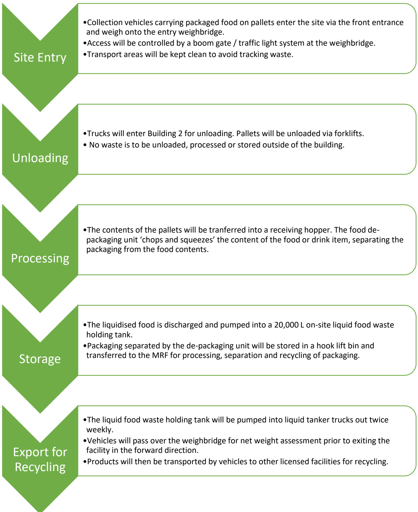
Figure 4.5. Process flow chart for the operation of the Packaged Food Recycling Plant.
