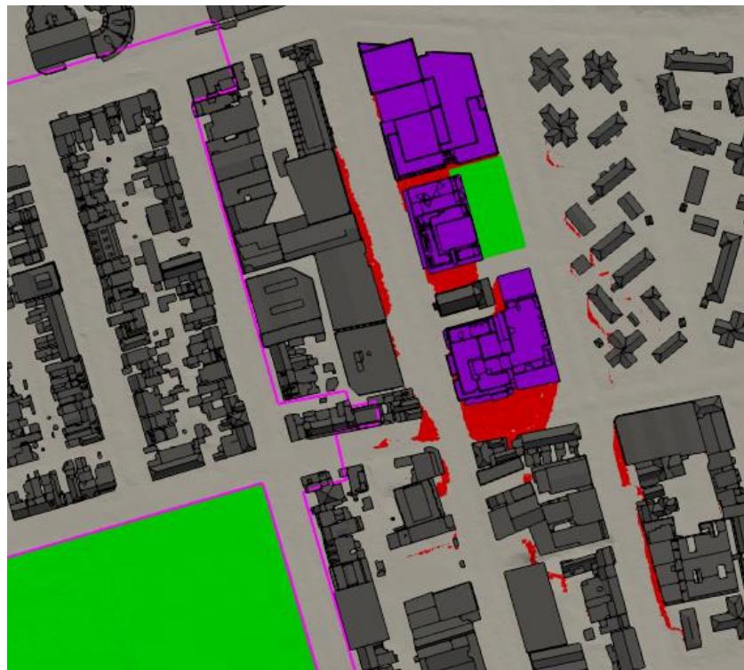
Figure 11 - Grade Level Areas Where Direct Solar Access is Reduced from At or Above 2 Hours to Less Than 2 Hours on 21 June
