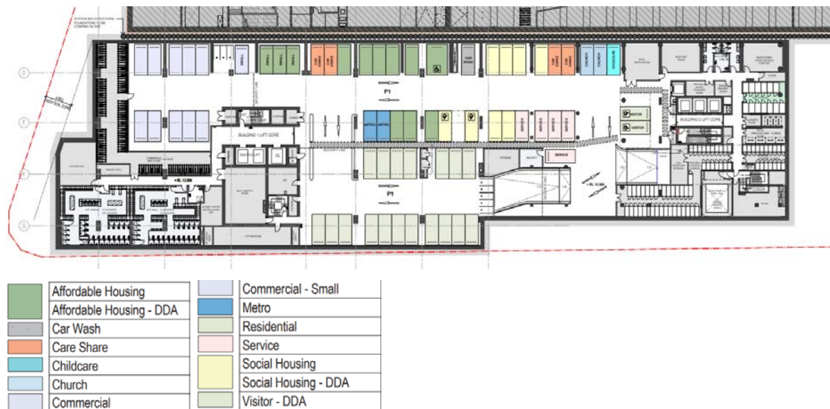
Figure 16 | Proposed layout for basement Level P1 (Source: Applicant's EIS)
