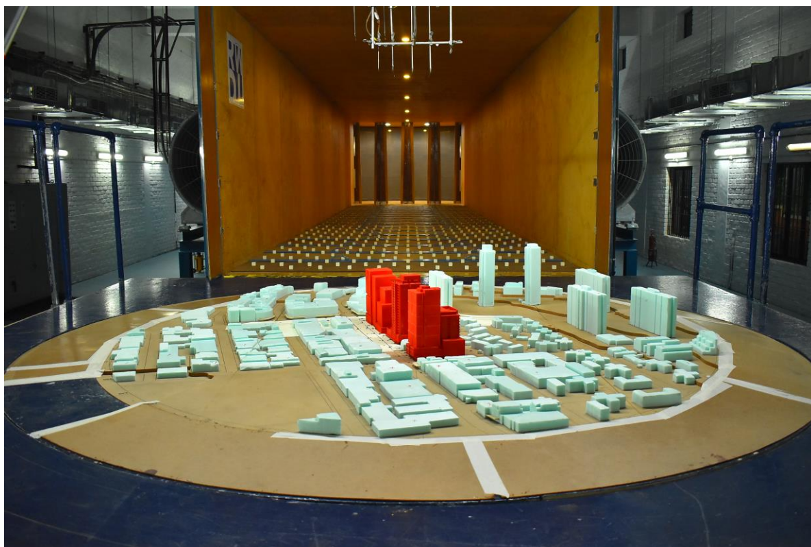
Figure A-1 – Wind Tunnel Model of Detailed Design (View from the South)
