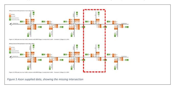
When the same analysis is carried out (outflow from one intersection should be close to the inflow into the next intersection), the same issue of disappearing vehicles arises. See Figure 6.
