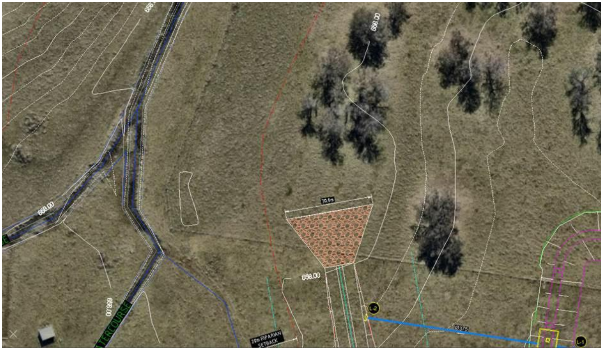
Figure 2. Concept drawing of a flow spreader at the downstream end of the proposed diversion channel (courtesy of Simon Haycock, AT&L).
