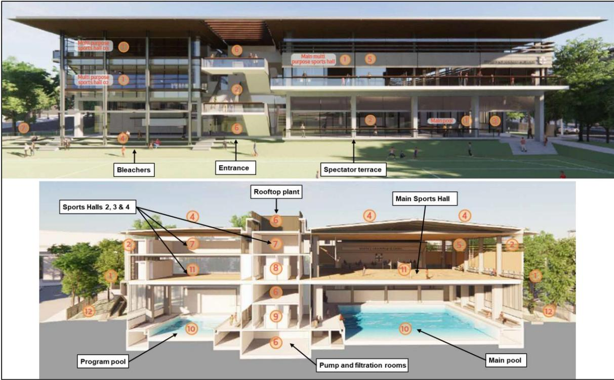
**Figure 11 | Building 1 northern elevation (top) and section through the building (bottom) (Source: Applicant's RtS 2021)**
