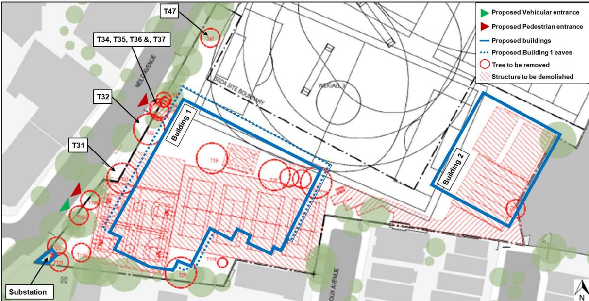
**Figure 42 |** Tree removal and demolition plan, approximate location of Building 1, 2 and the substation and proposed Neild Avenue entrances to Building 1 (Source: Applicant’s RtS 2021)
